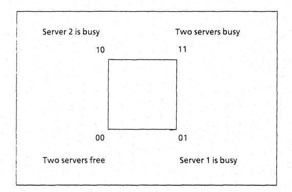
Only one-step transitions are allowed and the transition from one state to another occurs along the edges of the cube. The upward transitions are transitions that occur when a unit is dispatched and their rates can be calculated given the arrival rates of calls for service and the dispatch preferences for each atom. On the other
