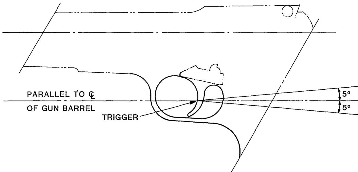
FIGURE 6. *Trigger pull test setup.*
