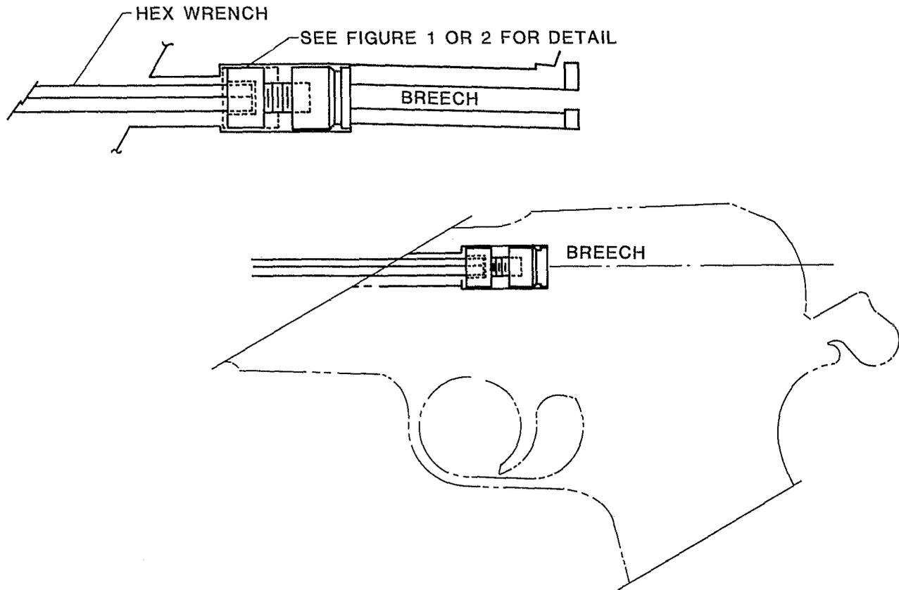
FIGURE 5. *Headspace gage usage.*
