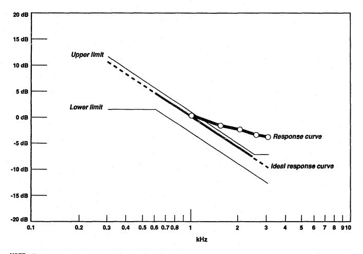
NOTE: Deviation could not be set to 1.0 kHz at 0.3 kHz and 0.5 kHz. Therefore, the audiofrequency response at these frequencies is not shown. Test Results (Continued)
