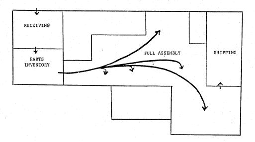
The layout shown above represents spatial relationships for proposed start-up products. An individual work station concept is proposed where one employee fully assembles the product from start to finish.
