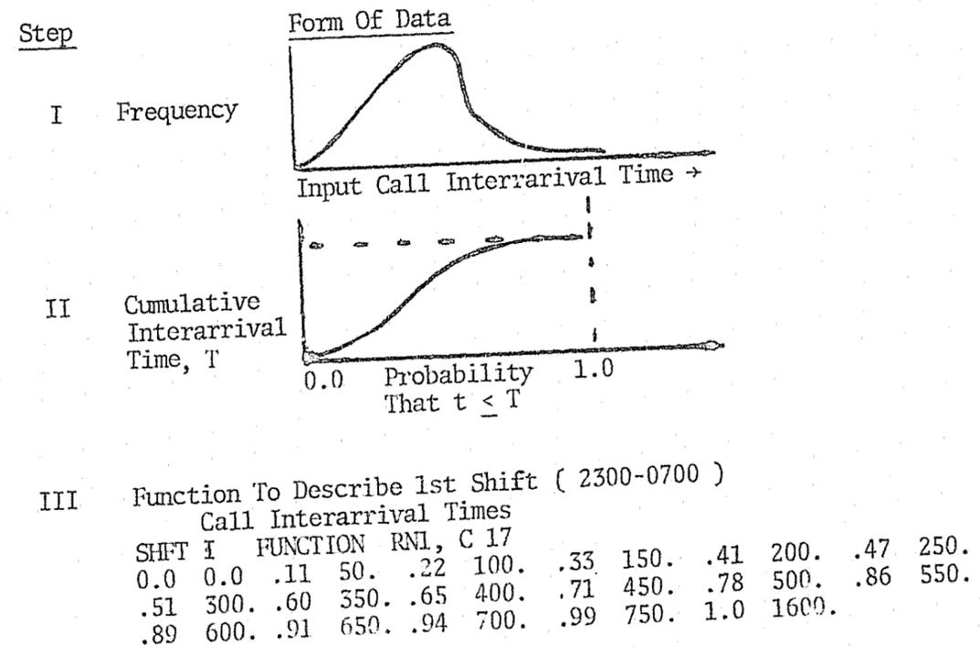
Figure 16 Steps In The Transformation Of Basic Statistical Data About The Command/Control Center Into Form Useable By The Computer Model
