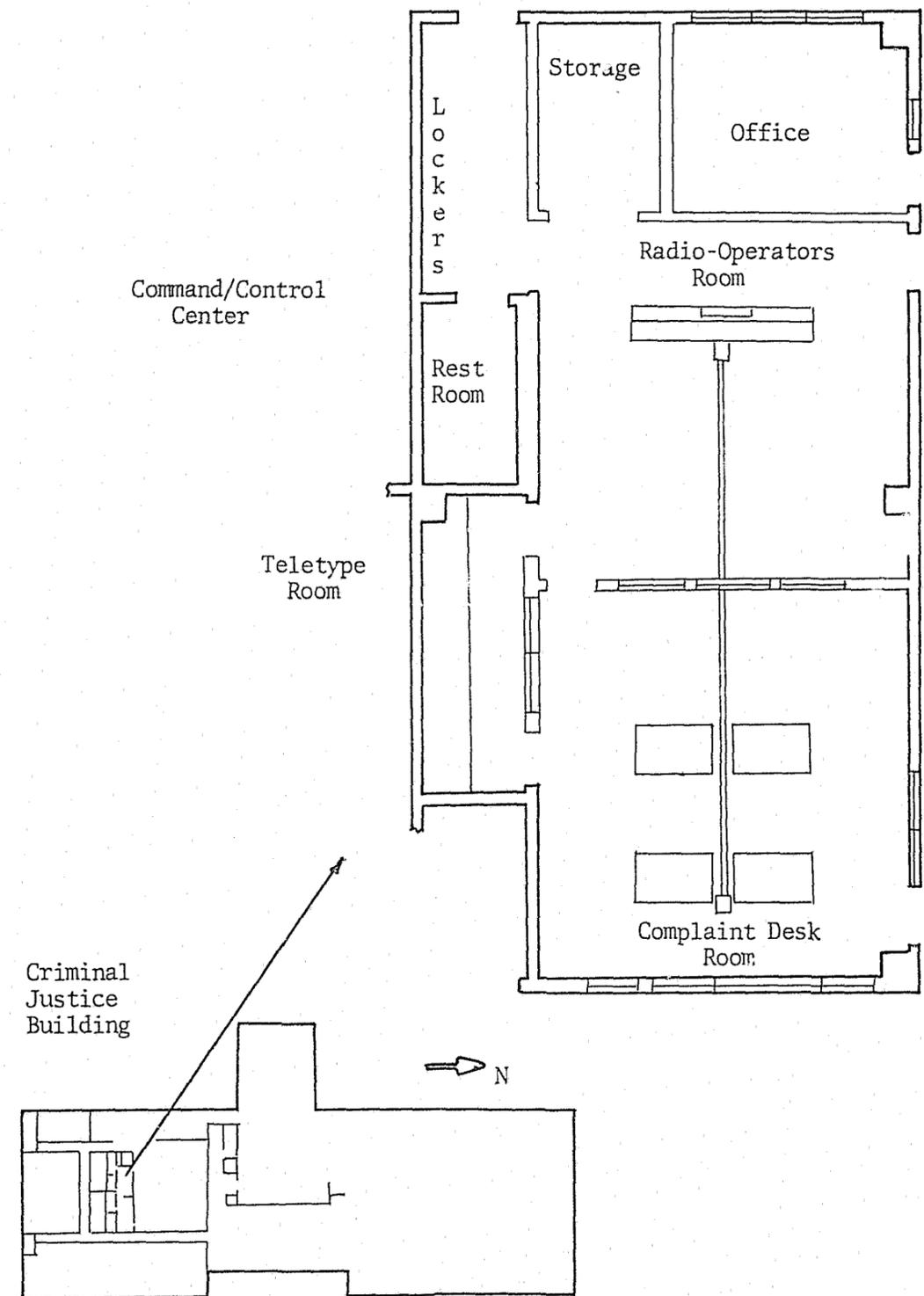
Figure 8 Showing The Three Work Rooms Of The Command/Control Center And Their Locations Within The Criminal Justice Building
