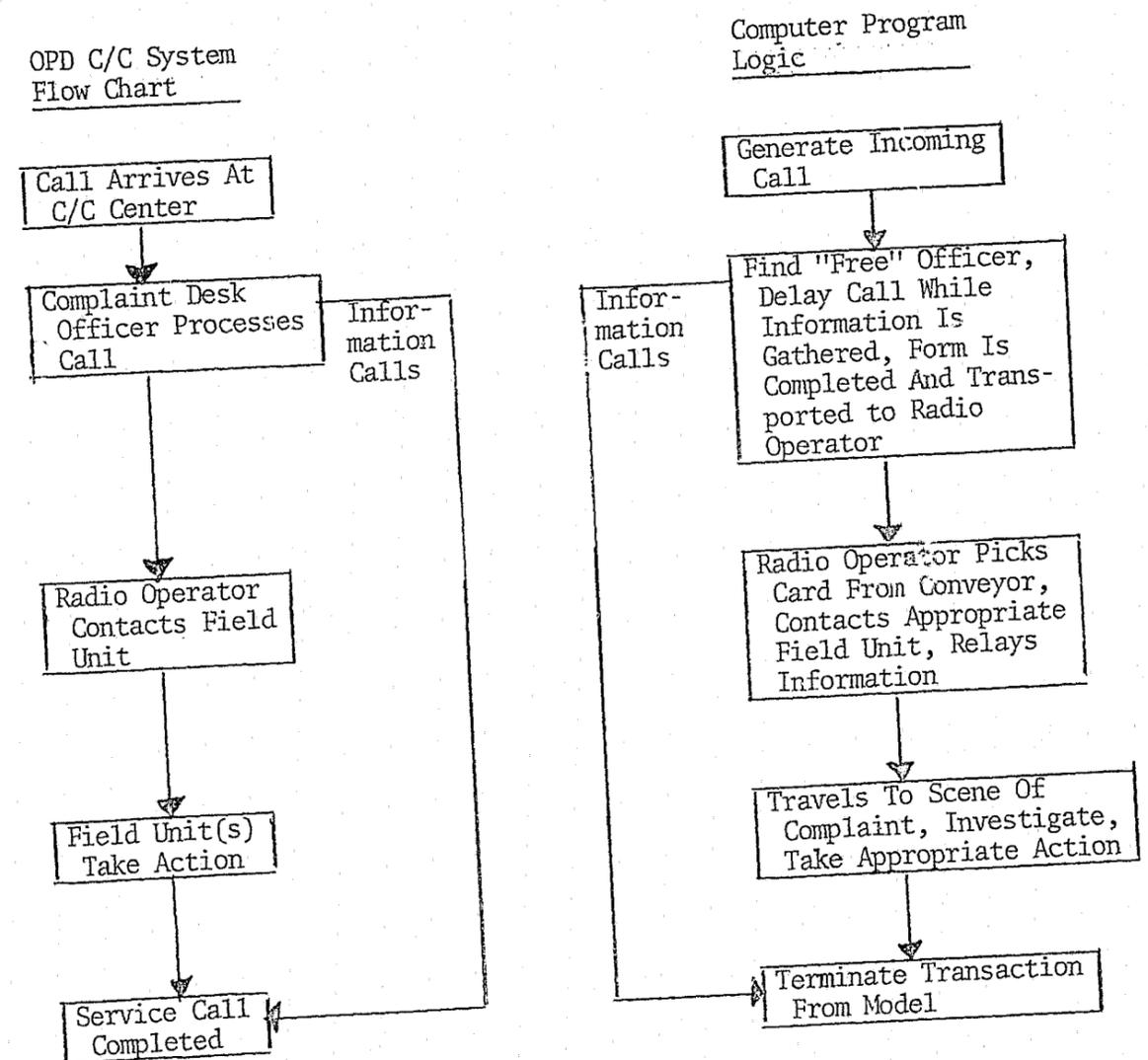
Figure 15 Shows Equivalence Of GPSS/360 Program Logic Blocks To Flow Chart Of Actual System.
