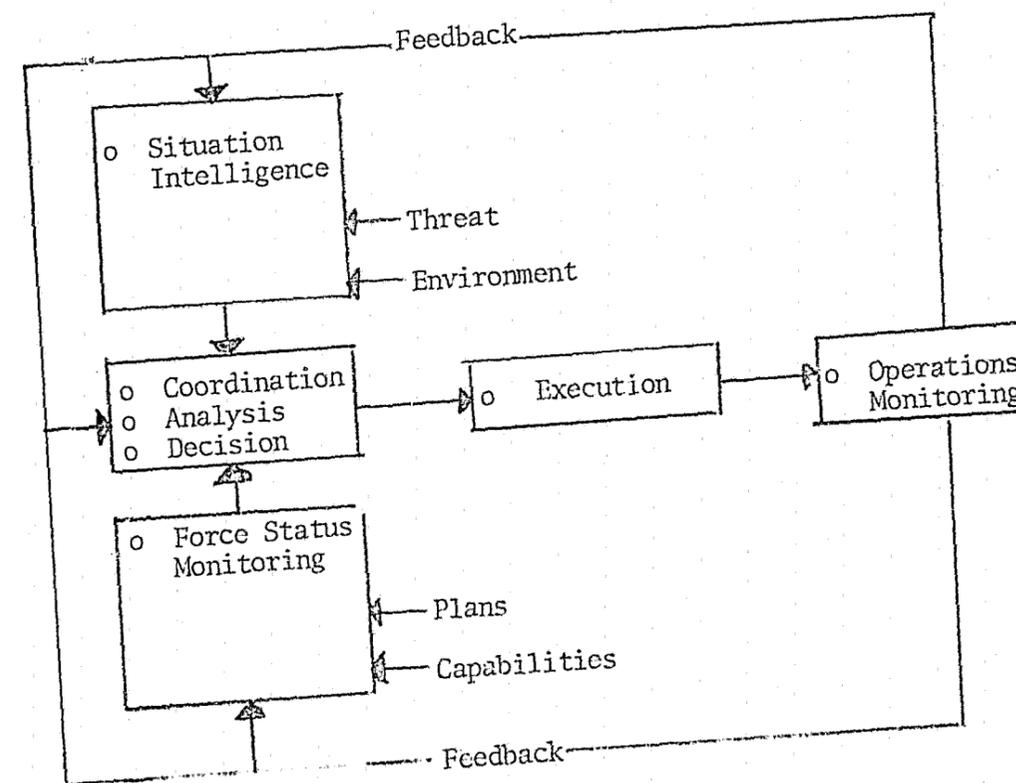
Figure 1 Functional Block Diagram Of Basic Command/Control Process Shows Its Dependency On A Closed Loop Feedback System.
