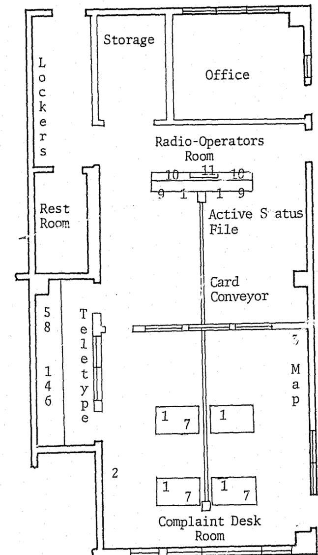
Figure 9 Showing Major Equipment Locations For Each Specialized Task Of Command And Control.
