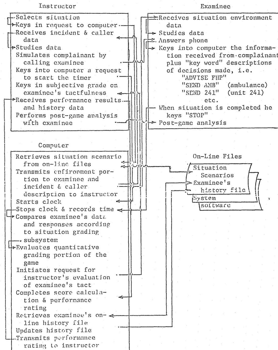
Figure 20 The Figure Above Shows the Logic Flow of the Computer Augmented Game Model
