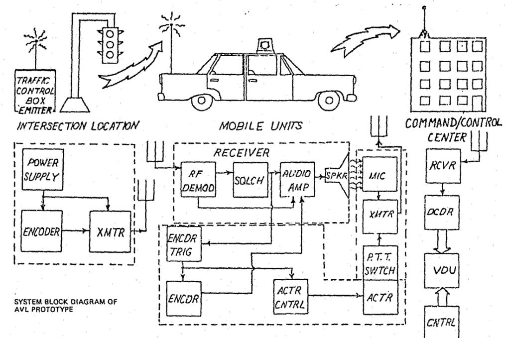
Figure 17 Block Diagram of the System
