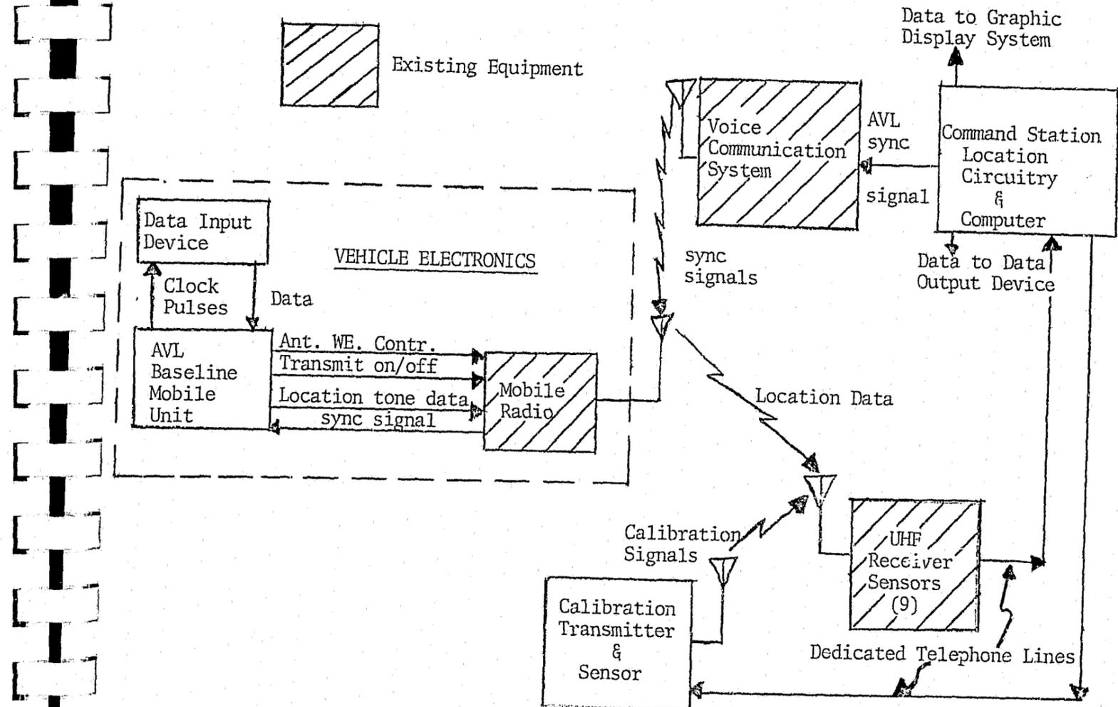
Figure 30 AVL System Block Diagram Shows Compatibility with Existing PREP System
