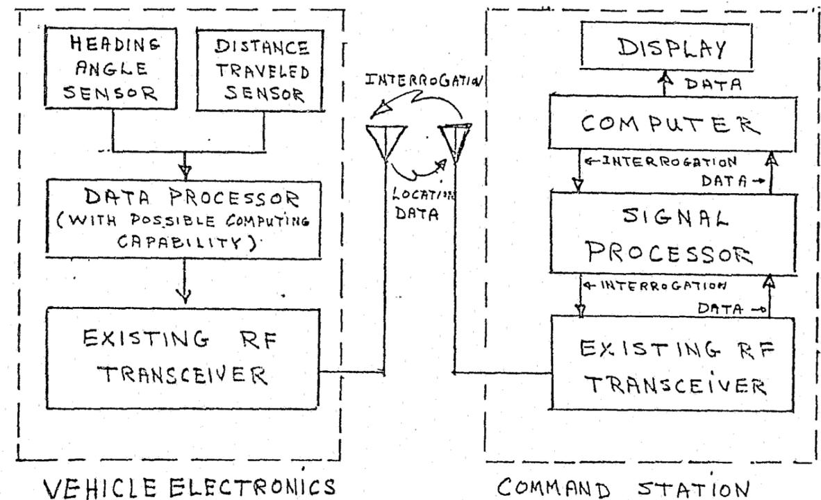
FIGURE 13 FUNCTIONAL BLOCK DIAGRAM OF DEAD RECKONING AVL SYSTEM SHOWING MAJOR COMPONENTS
