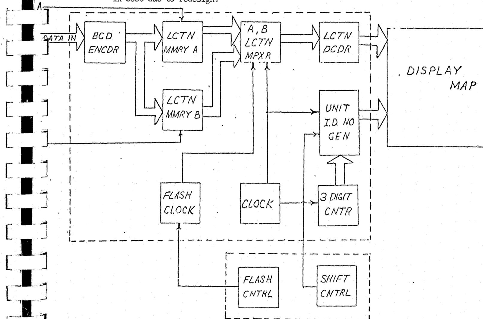
Figure 23 Visual Display System Block Diagram
