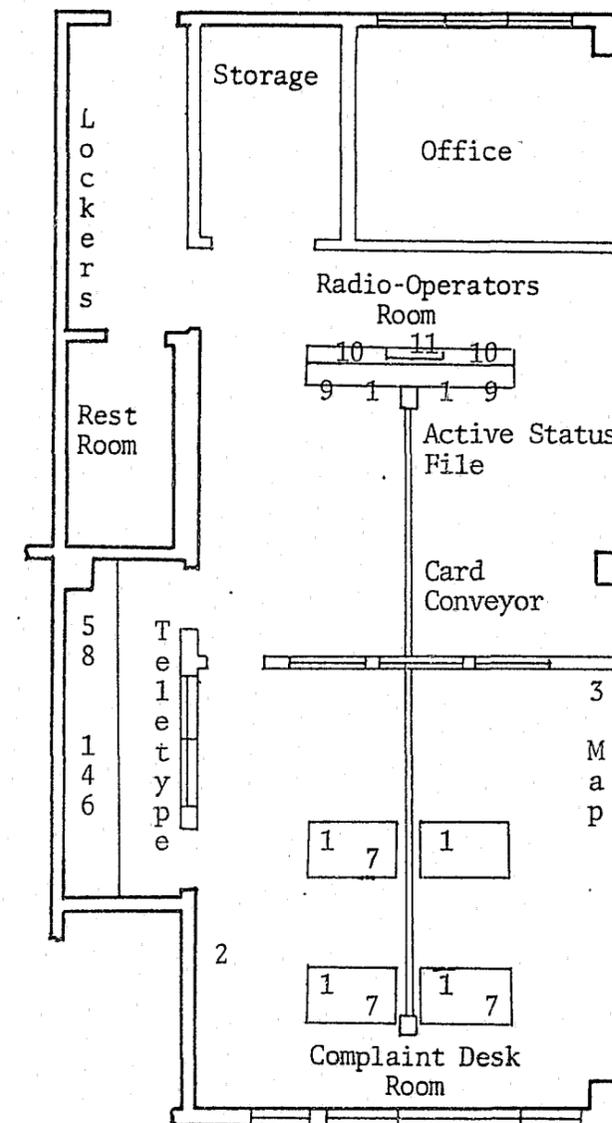
Figure 8 Major Equipment Locations For Each Specialized Task of Command/Control System At The Communications Center
