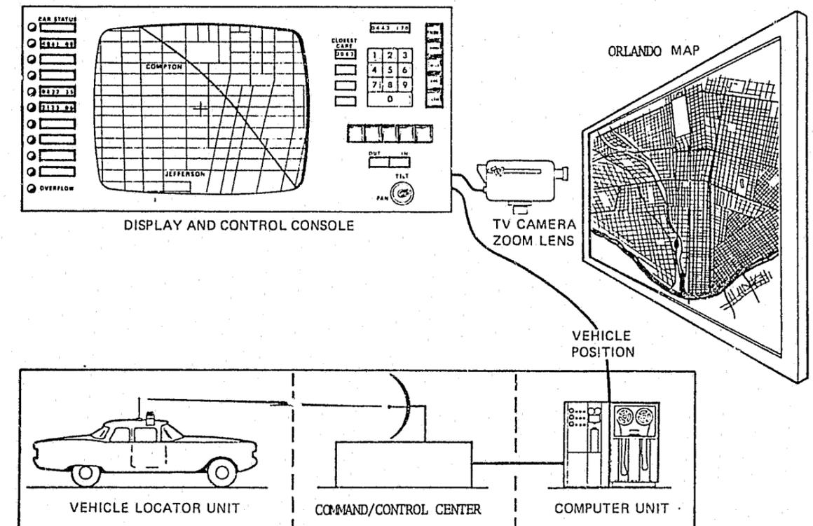
FIGURE 35 FLAIR SYSTEM CONCEPT SHOWS MAJOR FUNCTIONAL COMPONENTS AND THEIR INTERRELATIONSHIP
