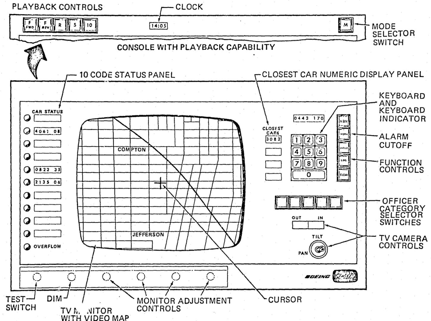
FIGURE 37 SITUATION DISPLAY AND CONTROLS
