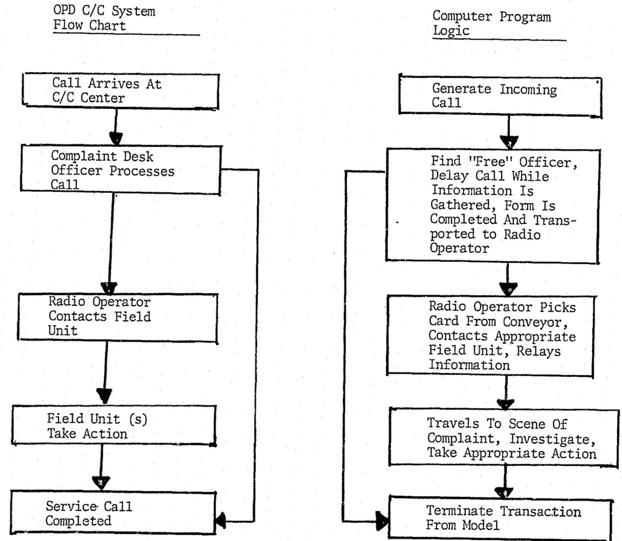
Figure 40 Shows Equivalence Of GPSS/360 Program Logic Blocks To Flow Chart Of Actual System
