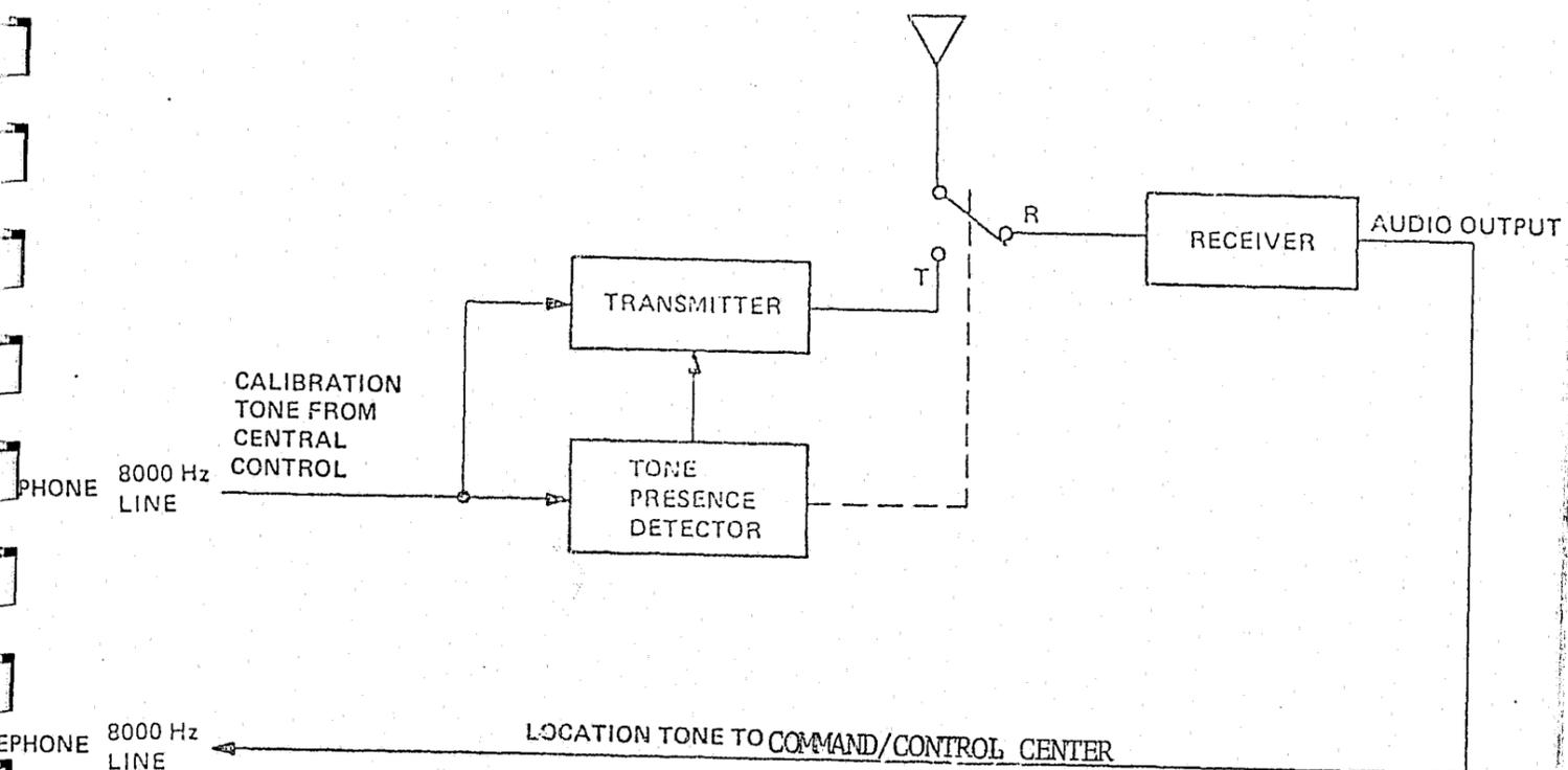
Figure 33 Combined Sensor-Calibration Station
