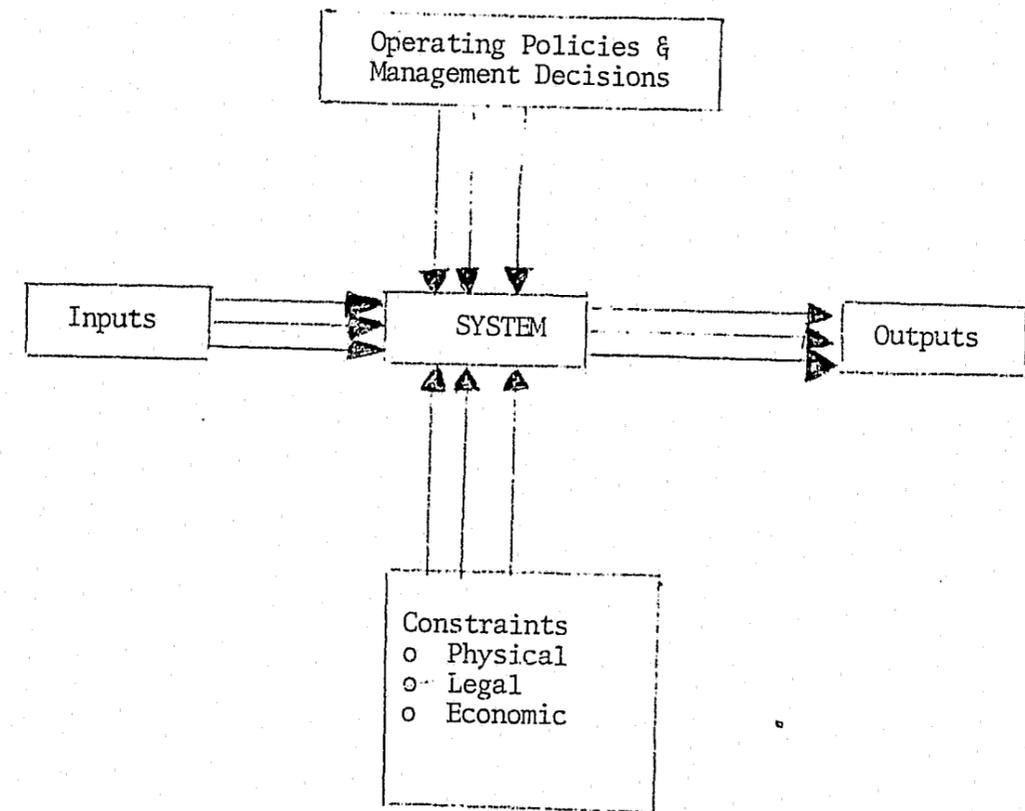
Figure 39 "Black-Box" Diagram Shows System Operating Environment Typically Consists Of Constraints, Controls and Inputs.
