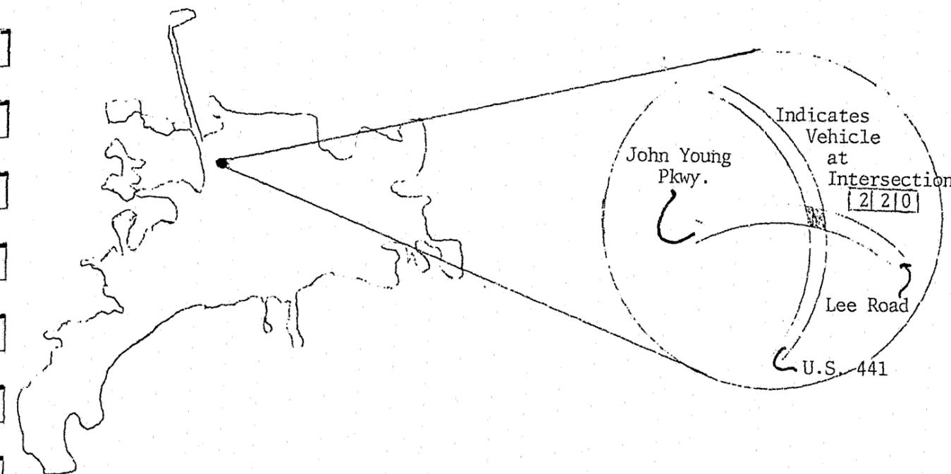
Figure 22 Typical Display Of Major Intersection Shows How Information Would Be Presented To Identify Patrol Vehicle And Its Location.
