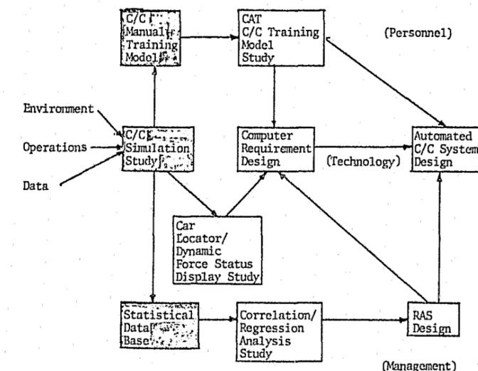
Figure 2: Logic Diagram Relating System Studies And Determination Of Design Requirements For Orlando Police Department Automated Command/Control System Identifies Three Major Areas Of Effort, Personnel, Technology and Management, Which Are Required.
