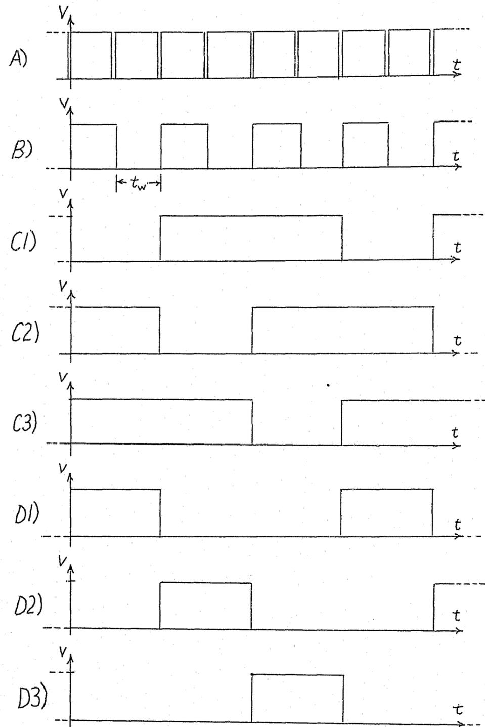
Figure 57: Pulse Trains: A) N74123 output, B) clock waveform, C) decoder/demultiplexer enabling waveforms, D) decoder/driver blanking waveforms.
