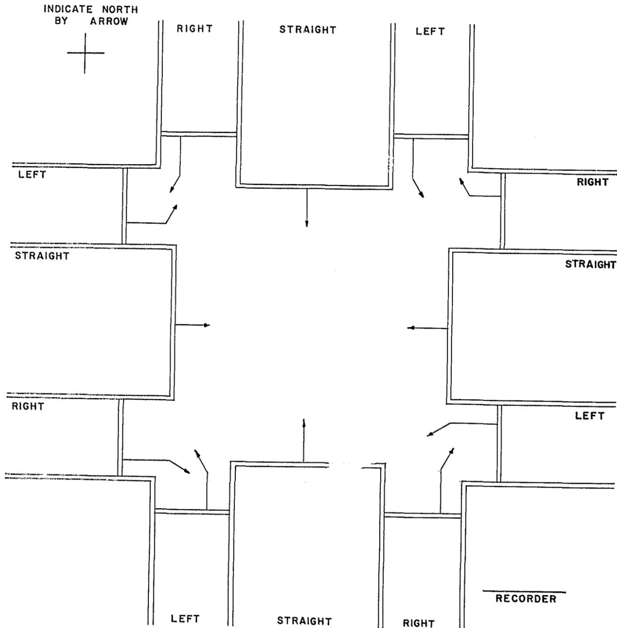
Figure 7-1. Vehicle volume field sheet.
