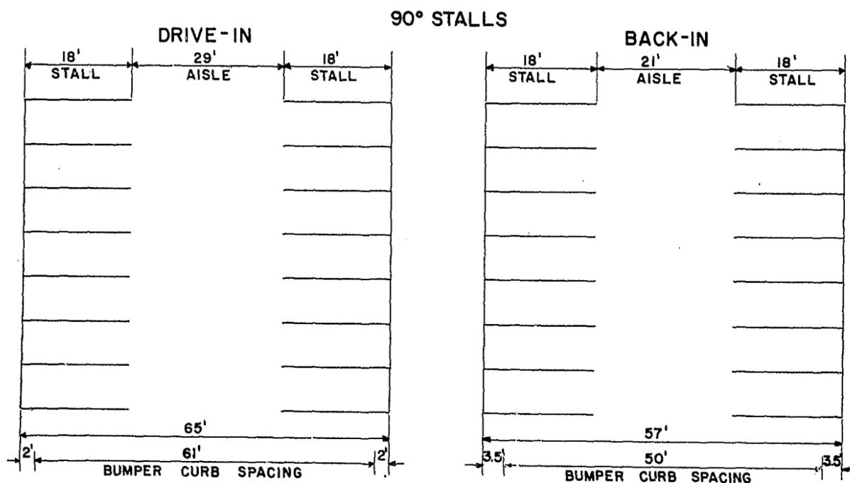
Figure 13-6. Minimum dimensions for parking area layout, 90° stalls.
