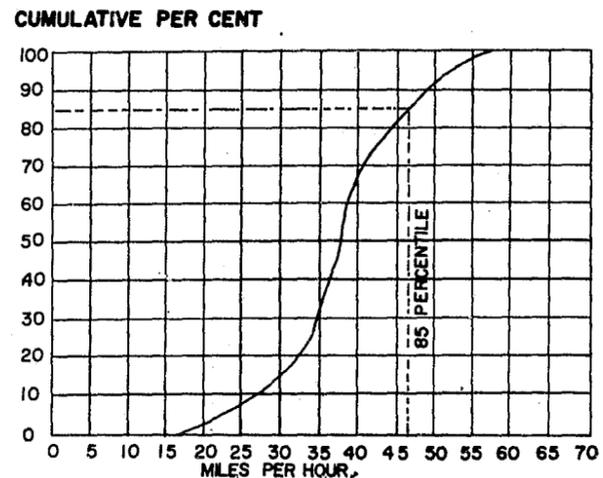
Figure 5-2. Speed accumulation chart.
