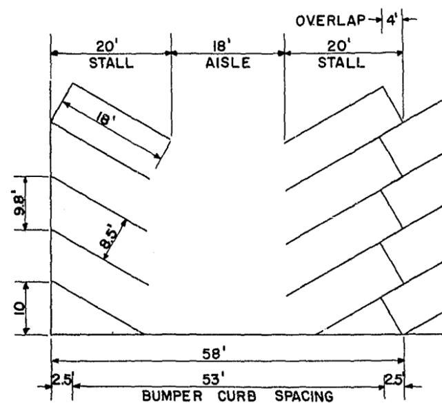
Figure 13-7. Minimum dimensions for parking area layout, 60° stalls.
