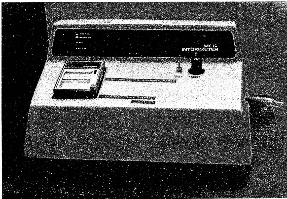
Figure 27. - Gas Chromatograph Intoximeter (GCI) for measuring blood alcohol levels
