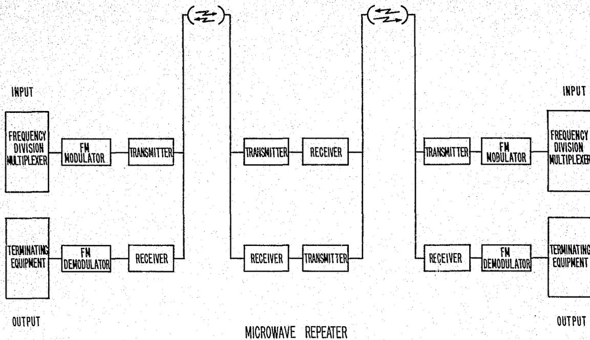
Figure 7—Block Diagram of a Microwave Repeater
