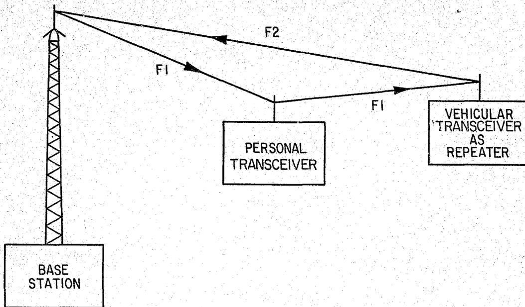
Figure 6—Block Diagram of a System Using the Vehicular Transceiver as a Repeater
