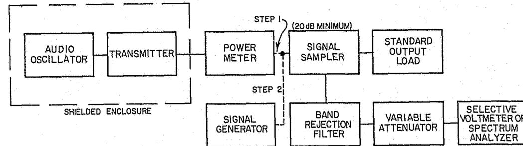
FIGURE 9. Block diagram for conducted spurious emissions at the antenna terminals.
