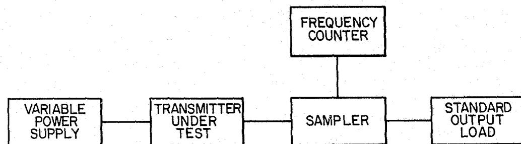
FIGURE 3. Block diagram for frequency stability measurement.
