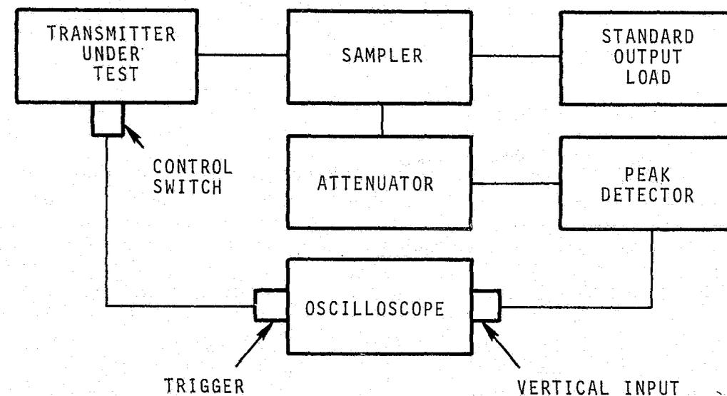
FIGURE 5. Block diagram for carrier attack time measurement.
