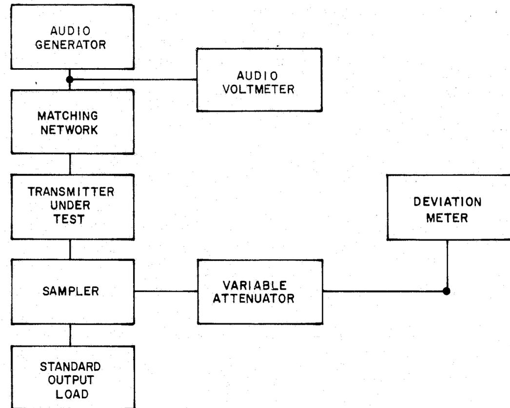
FIGURE 7. Block diagram for audiofrequency response measurement.
