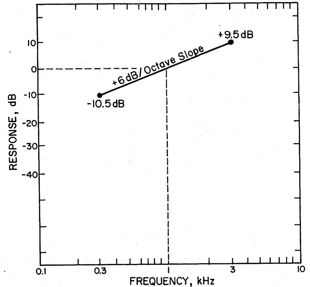
FIGURE 1. Audiofrequency response characteristics of fixed and base station FM transmitters.
