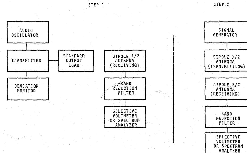
FIGURE 11. Block diagram for radiated spurious emission measurements.
