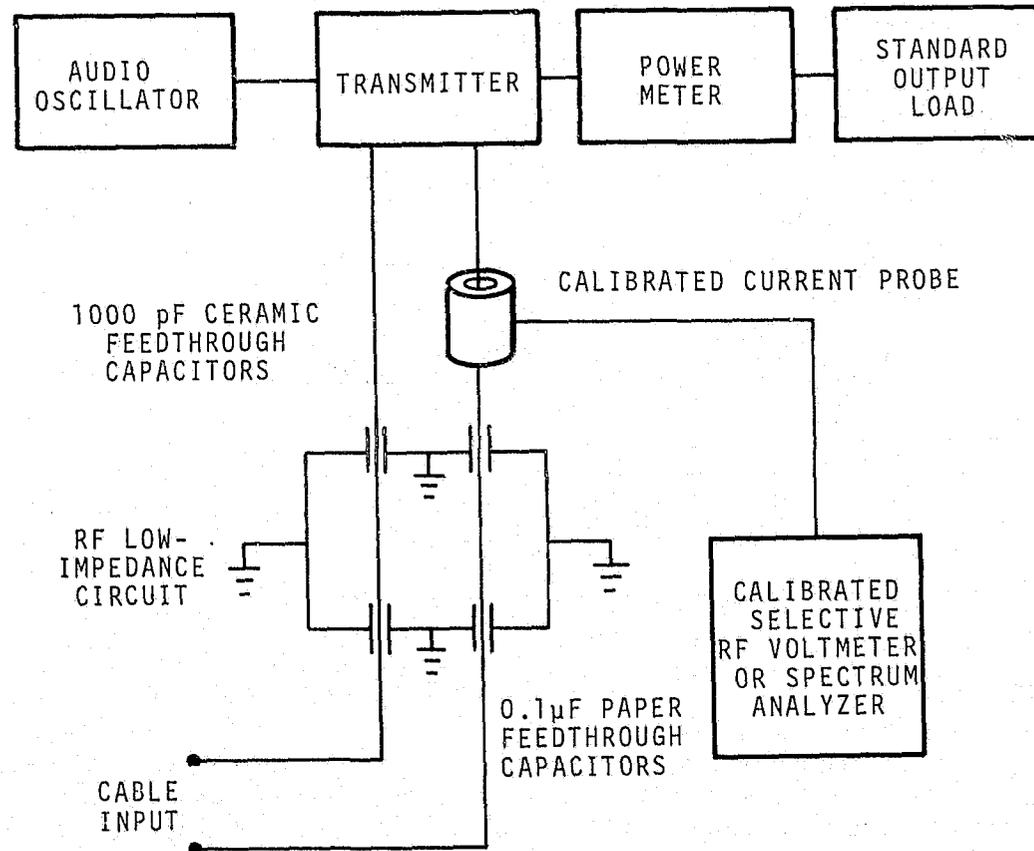
FIGURE 10. Block diagram for conducted spurious emissions measurements on cables.
