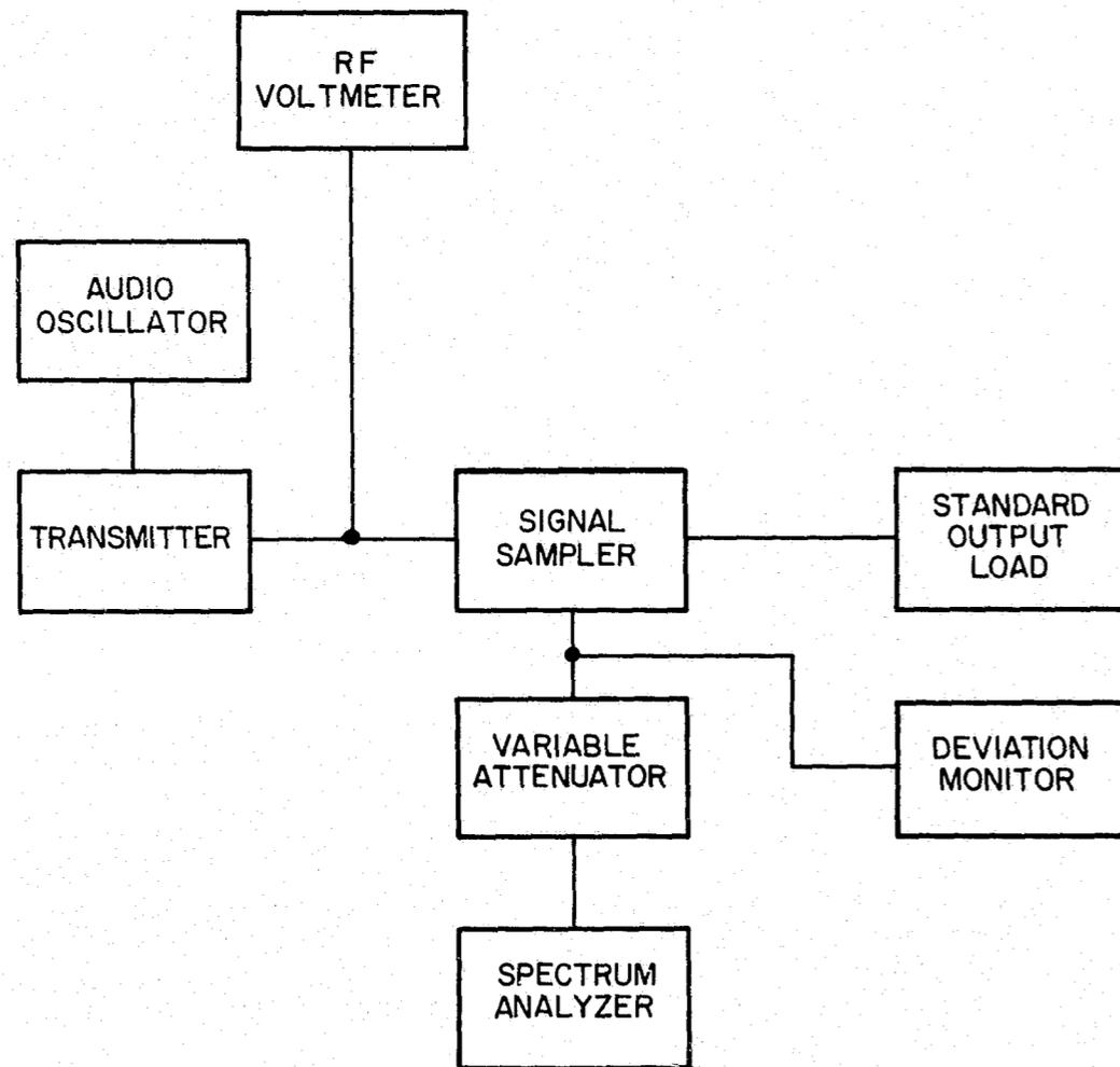
FIGURE 11. Block diagram for sideband spectrum measurement.
