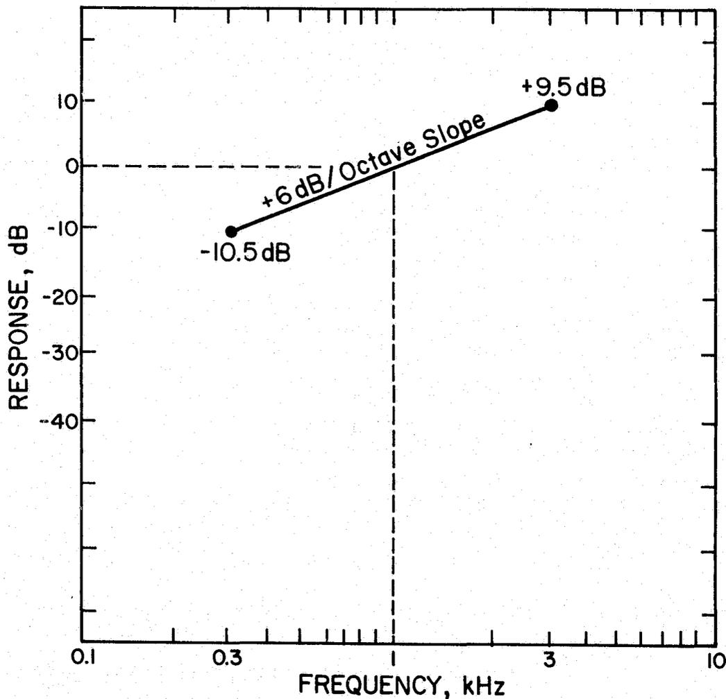
FIGURE 1. Audiofrequency response characteristics of mobile FM transmitters.
