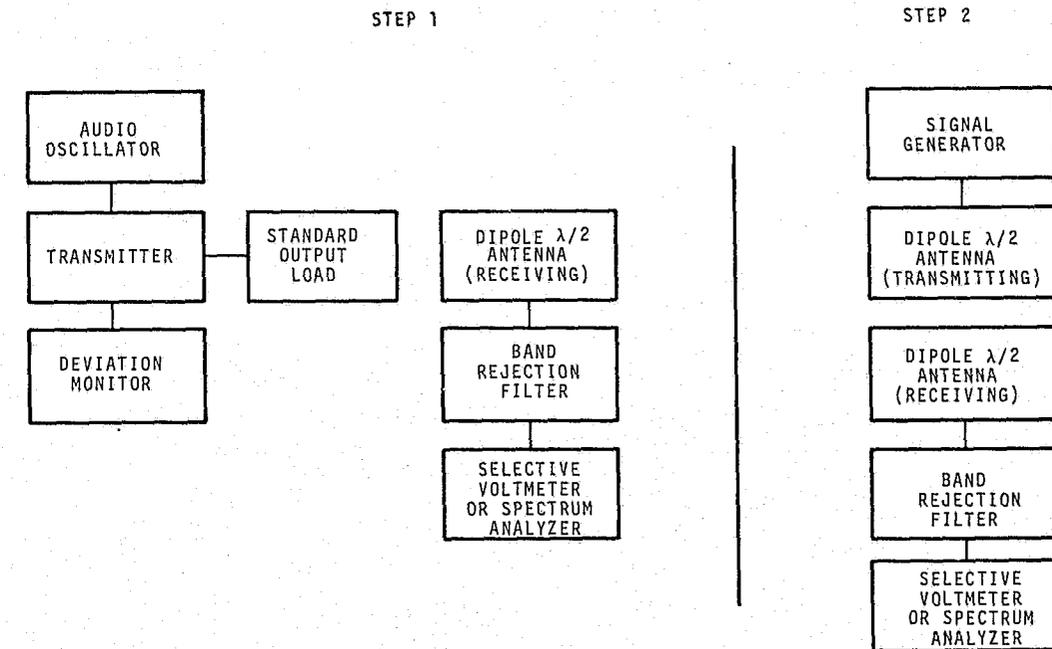
FIGURE 10. Block diagram for radiated spurious emission measurements.
