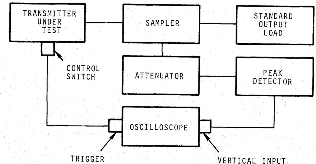
FIGURE 5. Block diagram for carrier attack time measurement.
