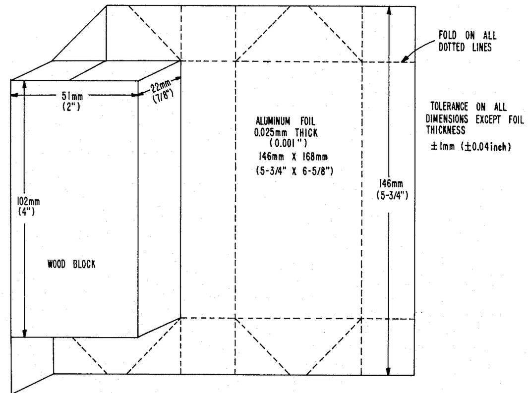
FIGURE 3. Foil Package Test Object
