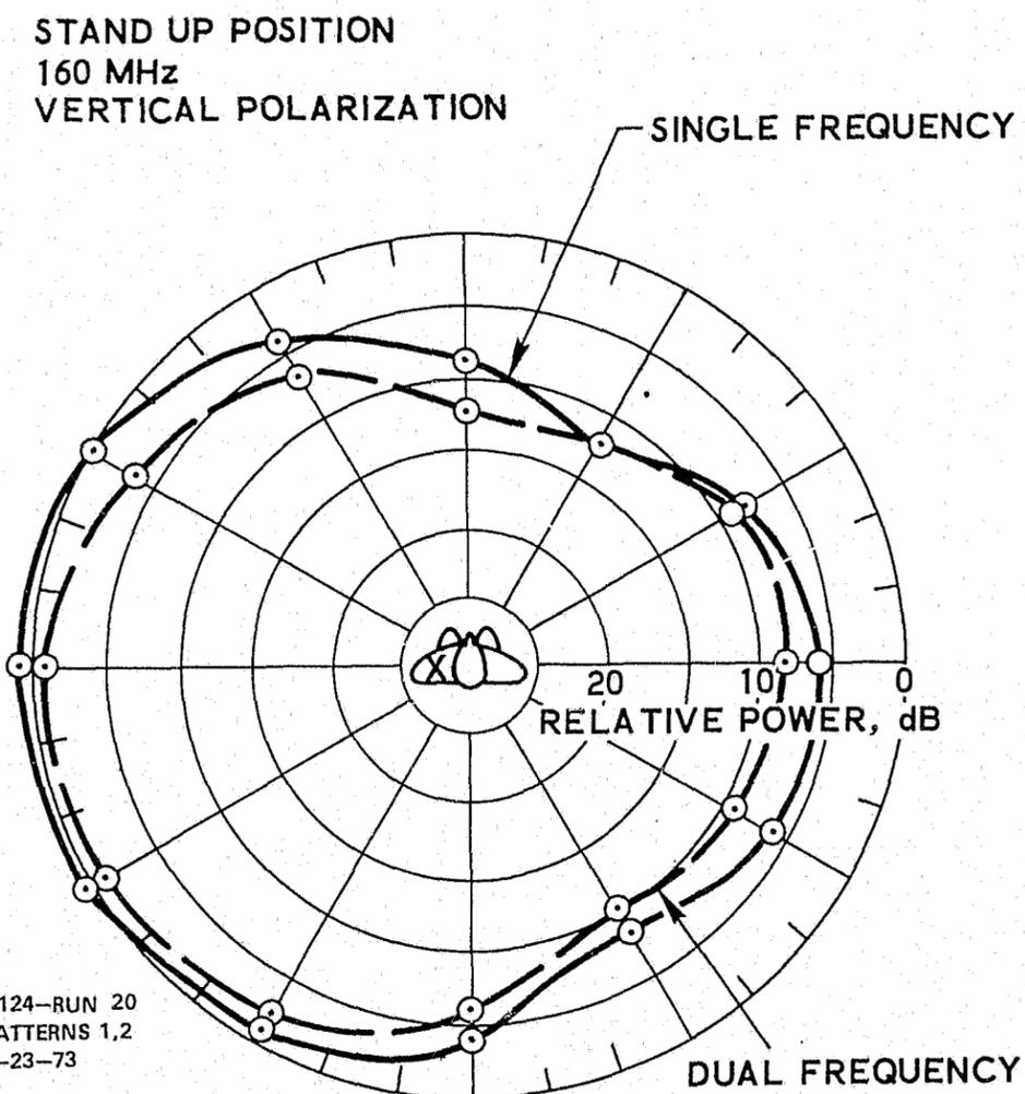
Fig. 3-22. Radiation Pattern of Shoulder-Mounted, Dual-Frequency Loop with Relay Switch.
