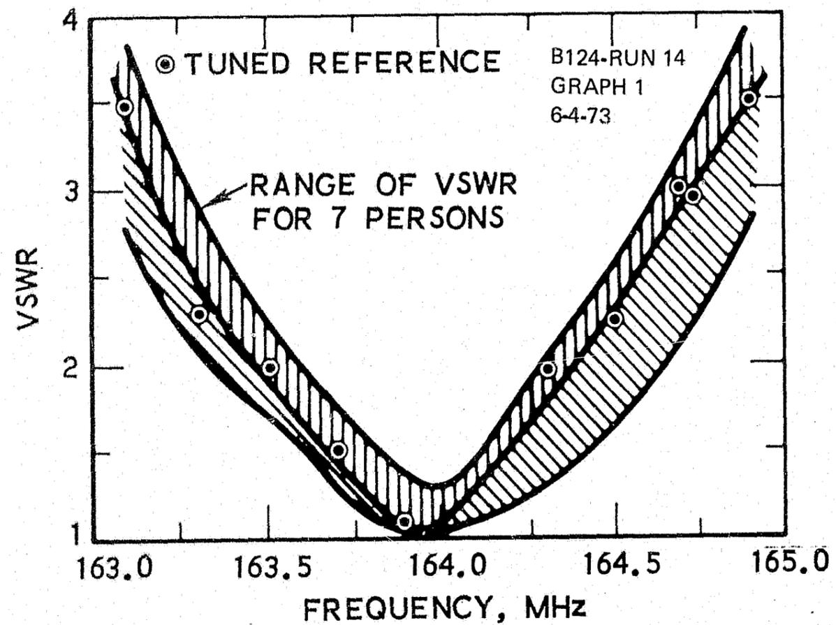
Fig. 3-15. Comparison of VSWR Characteristics of a Shoulder-Mounted Antenna on Different Persons.
