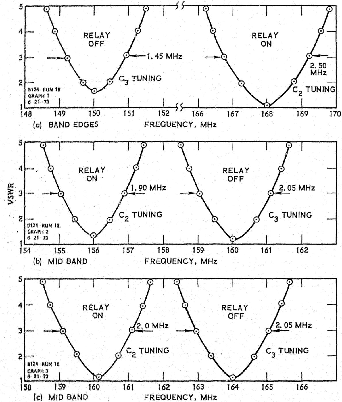
Fig. 3-21. VSWR of Dual-Frequency Loop (No. 14) with Reed Relay Switch.
