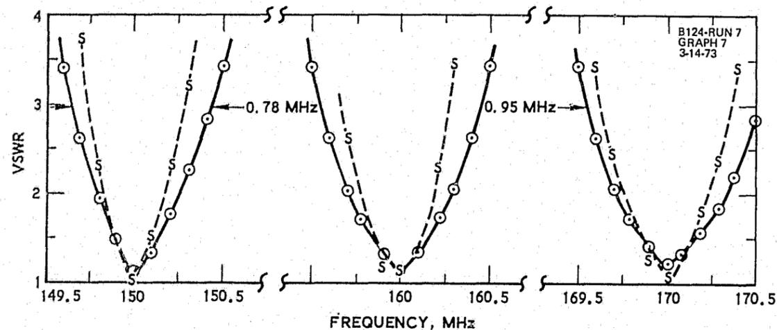
ANTENNA No. 5 AND 5S, 3-1/2 TURNS, 1/4 in. TUBING AND FLAT STRIP CONDUCTORS
