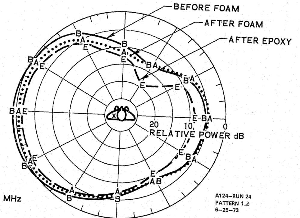
Fig. 3-25. VSWR and Radiation Patterns of a Multiturn Loop Between Each Fabrication Procedure.
