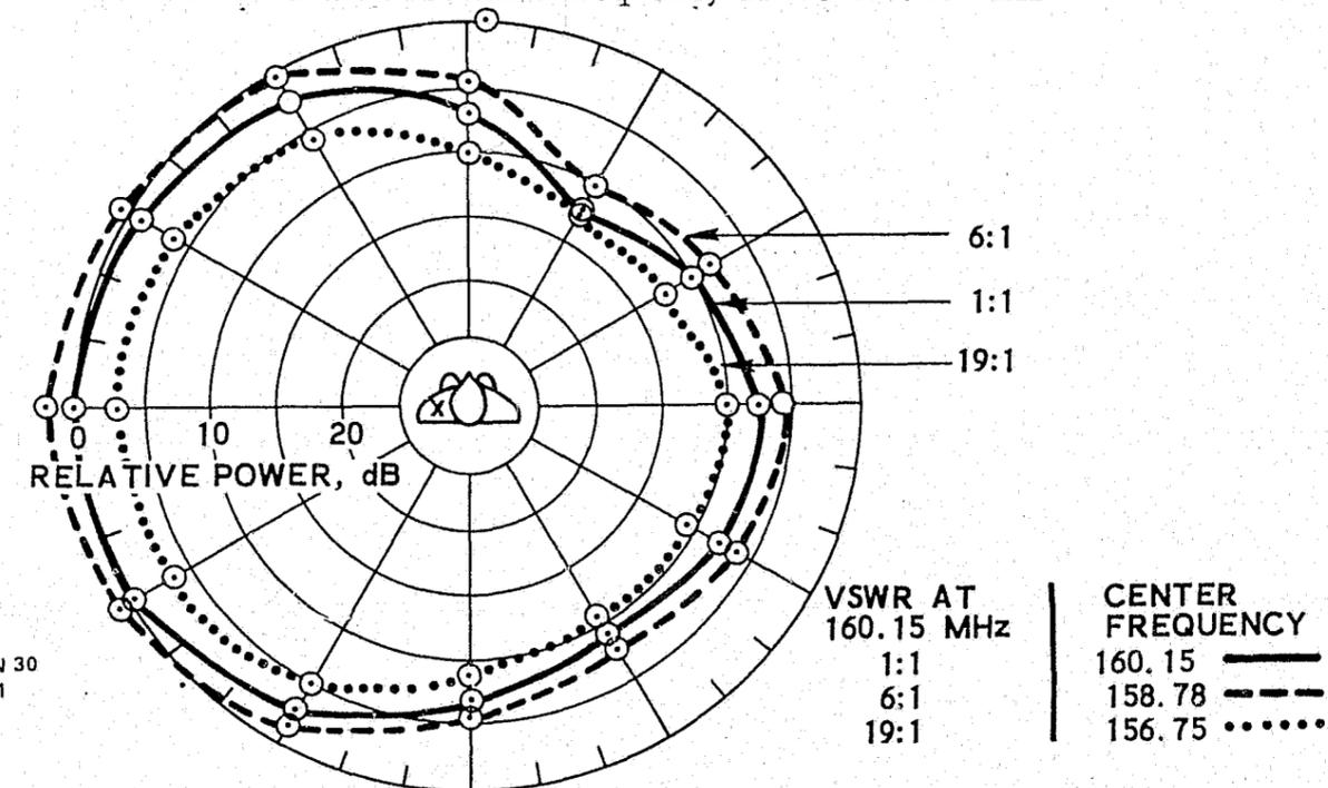
b. Patterns with resonant frequency below 160.15 MHz
