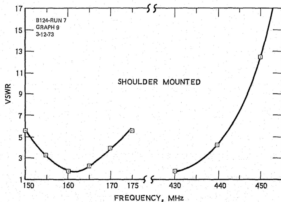
Fig. 3-3. VSWR Characteristics of a 6.6-in., Shoulder-Mounted Whip.
