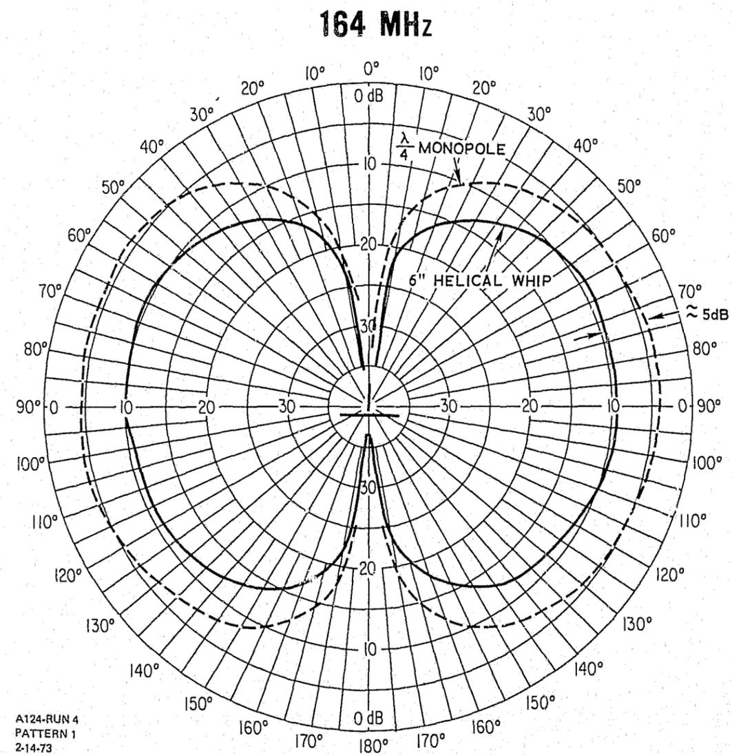
Fig. 3-1. Measured Radiation Patterns of a 6.6-in. Length Whip and  $\lambda/4$  Monopole Mounted on a 36-in. Diam Ground Plane.
