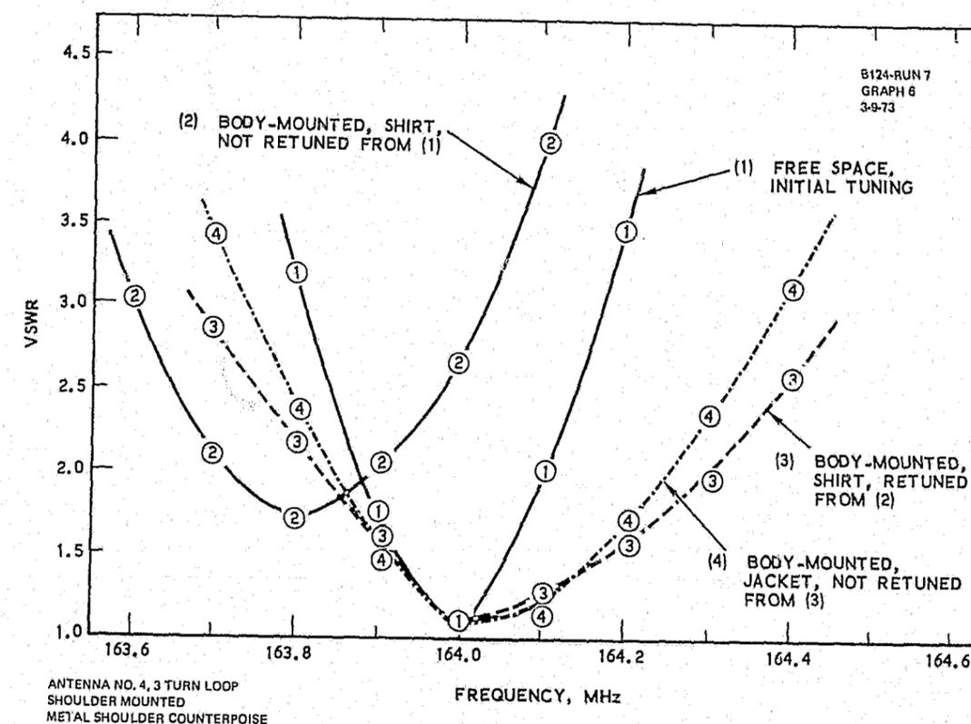
Fig. 3-13. Effects of Body and Clothing Upon the VSWR Characteristics of a Shoulder-Mounted Multiturn Loop.
