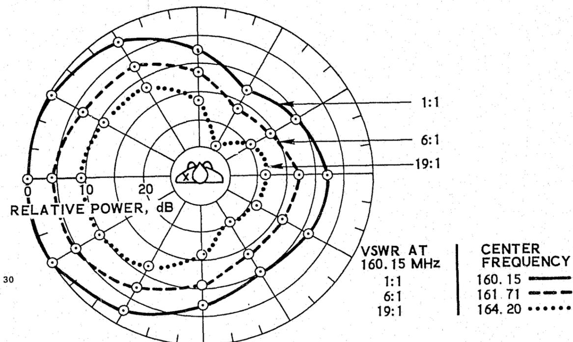
a. Patterns with resonant frequency above 160.15 MHz
