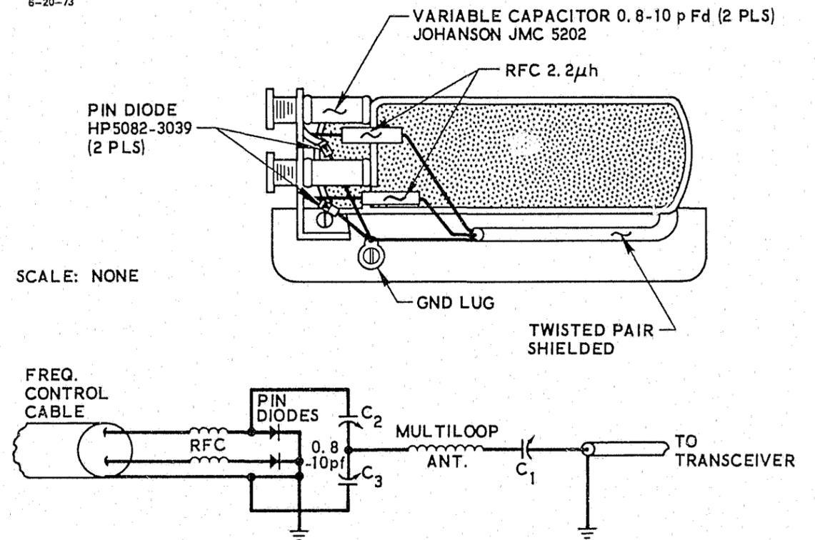
Fig. 3-24. Dual-Frequency Antenna with PIN Diode Switching
