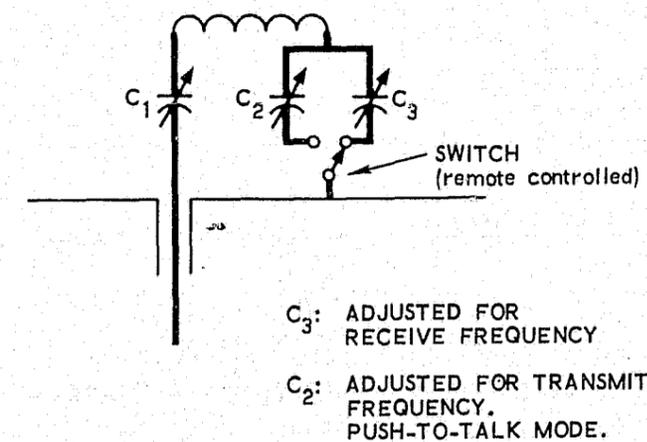
Fig. 3-19. Dual-Frequency Multiturn Loop Schematic.
