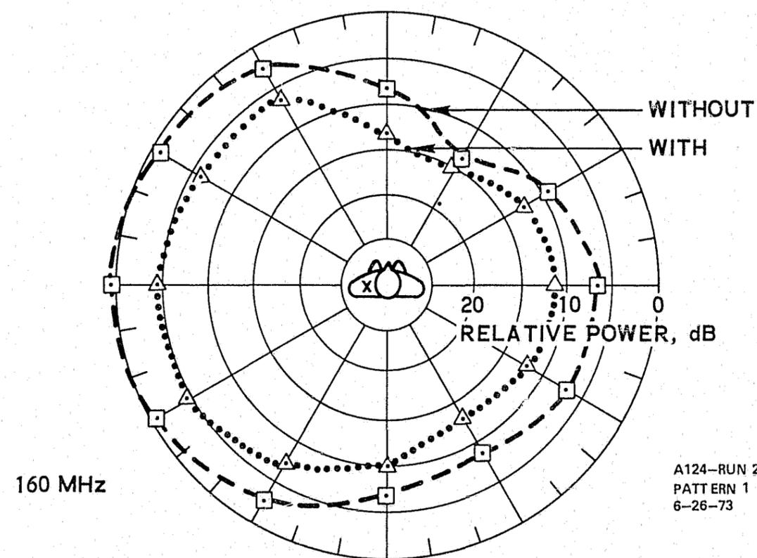
Fig. 3-14. Radiation Patterns of Shoulder-Mounted Antenna (8F) With and Without Heavy Leather Jacket.
