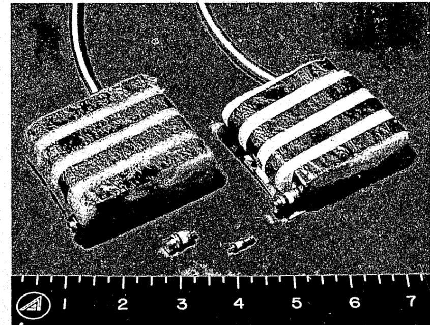
Fig. 2-3. Engineering Model of Multiturn Loop, Antenna No. 8F.
