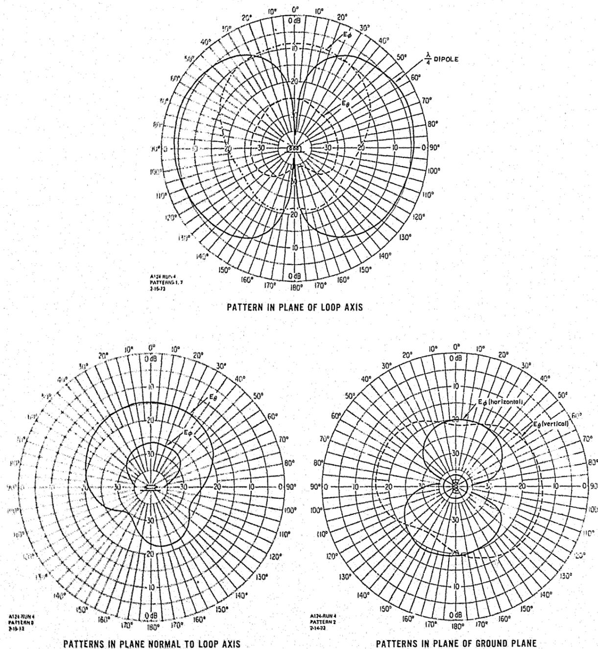
Fig. 2-5. Principal Plane Patterns (164 MHz) of Multiturn Loop Mounted on a 36-in. Diam Ground Plane.
