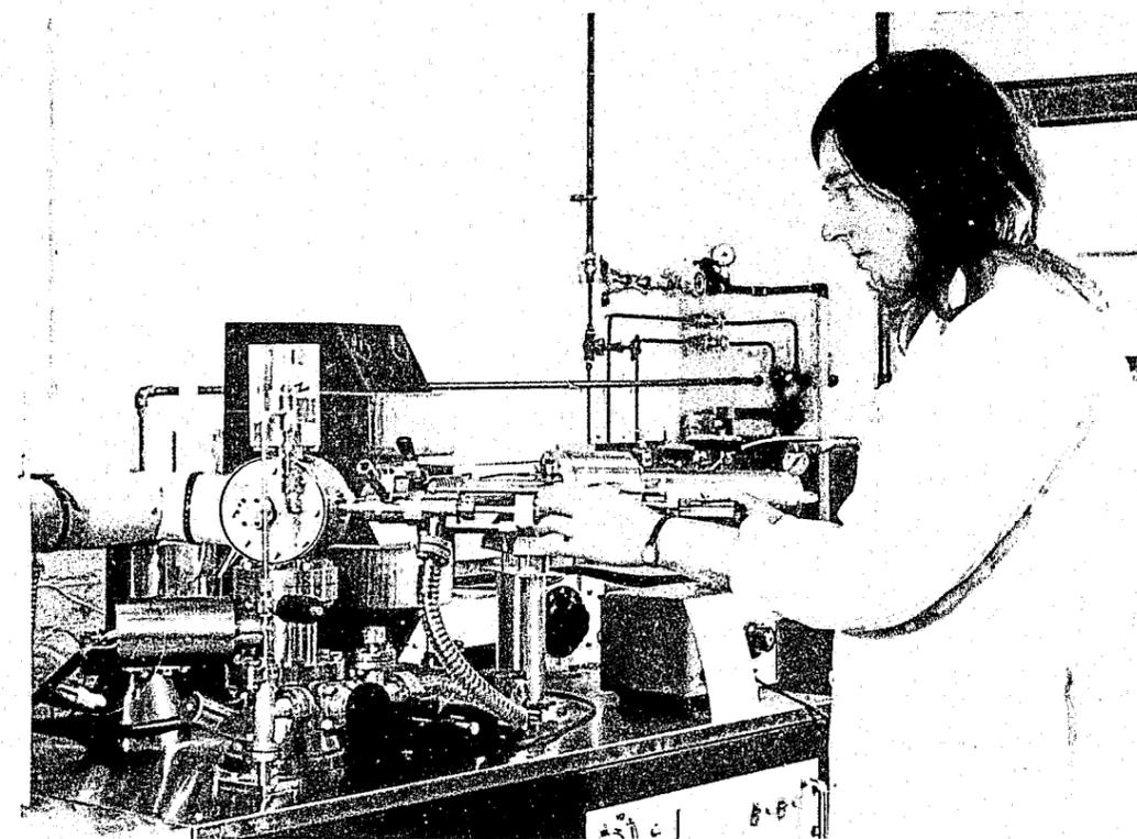
The Micromass 12 low resolution organic mass spectrometer, with a coupled GC system facility.
