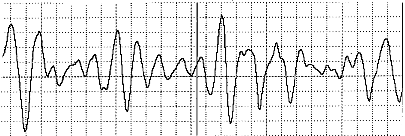
Figure 4. Radar cardiogram of subject 2 showing the differences in the heartbeat signature between test subjects.
