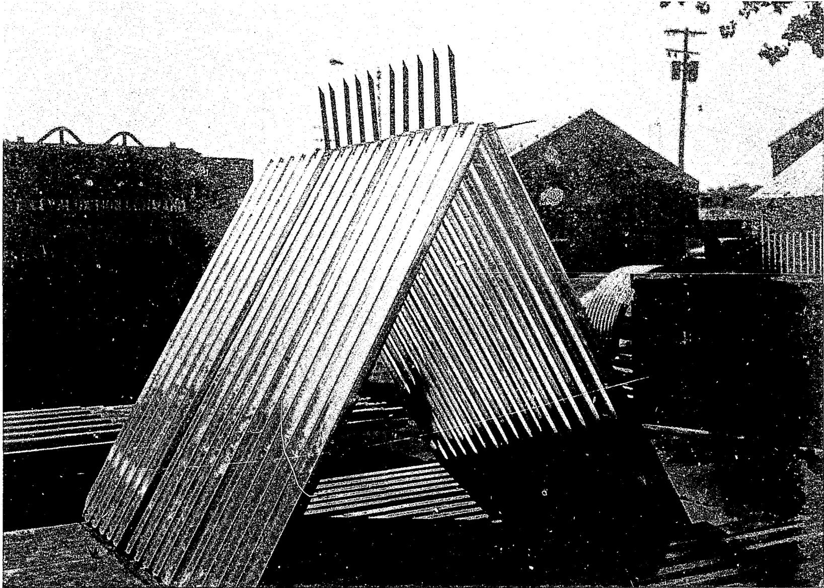
Figure 5. Alternate Riot Barrier Concept with Steel Spiked Apex.
