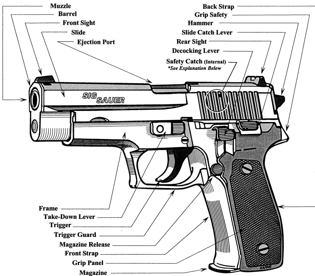
\* The Safety Catch is an internal design and locks the firing pin until the trigger is intentionally pulled which automatically releases the safety mechanism to initiate the firing sequence.
