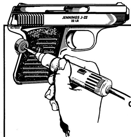
**Hand-held Motorized Grinding Wheel**
