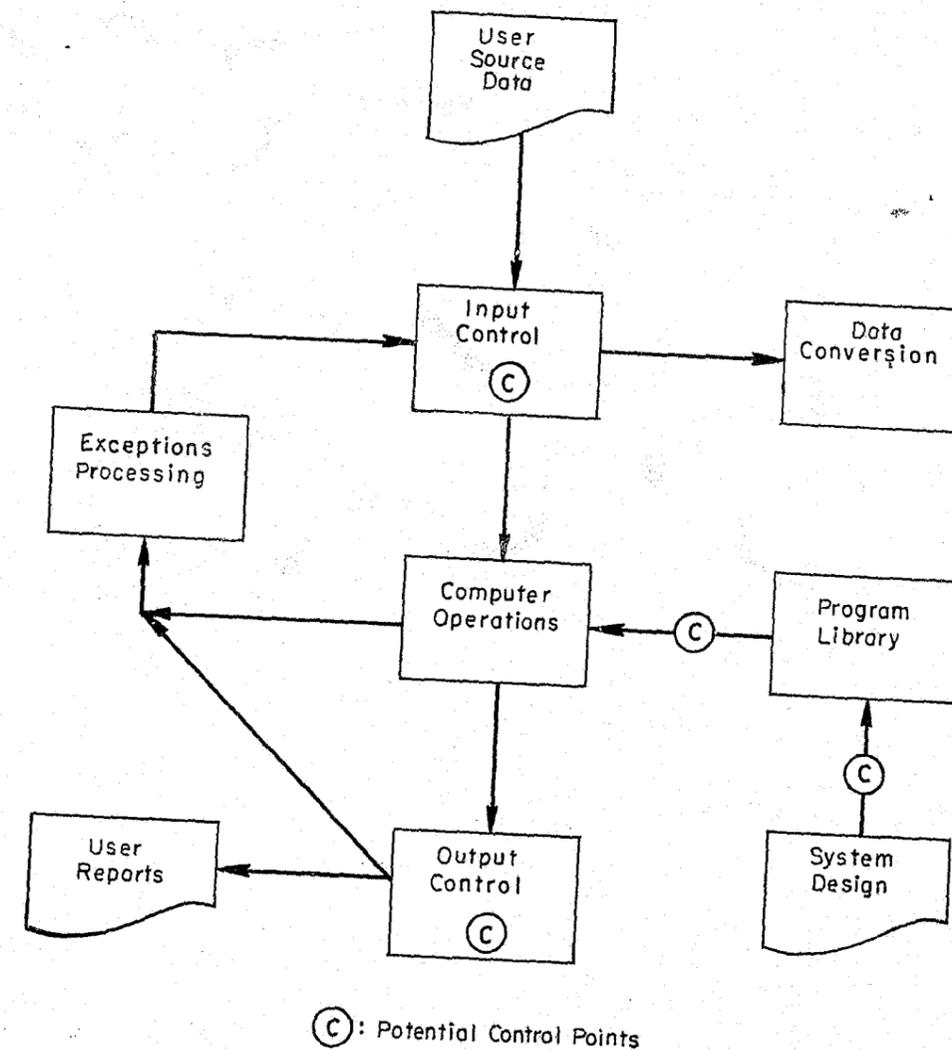
FIGURE 16. Work flow and control points.
