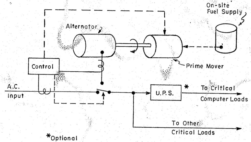
FIGURE 10. UPS with on-site generation.
