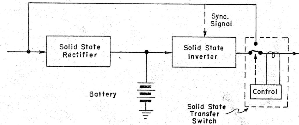
FIGURE 8. UPS with transfer switch.
