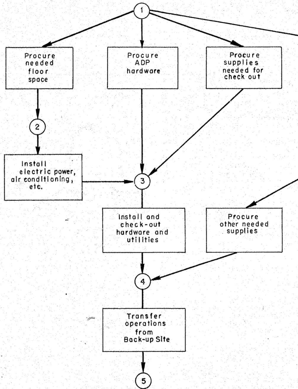
FIGURE 20. Simplified PERT diagram of ADP facility reconstruction.
