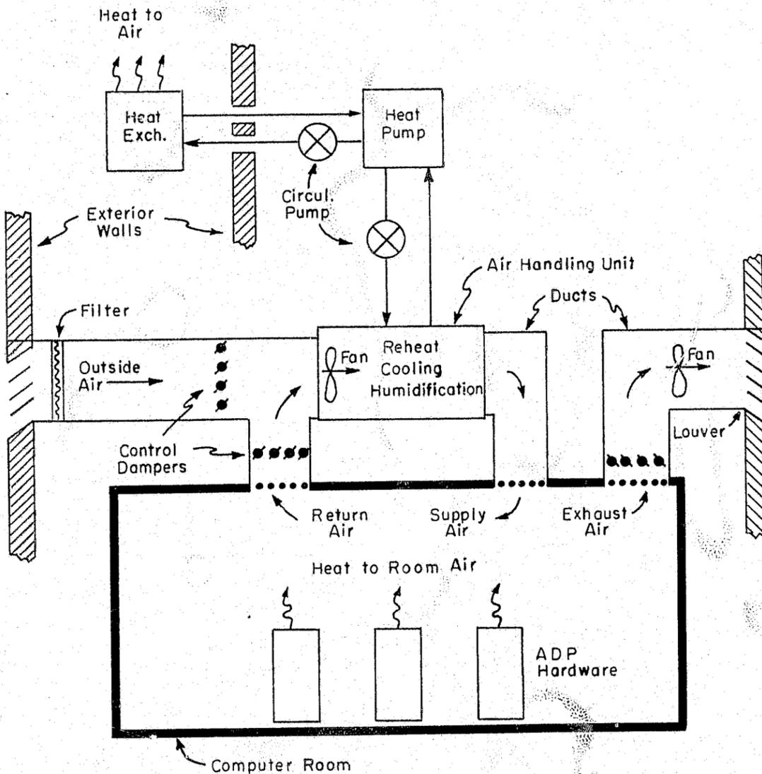
FIGURE 13. Cross-sectional schematic diagram of a typical air conditioning system.
