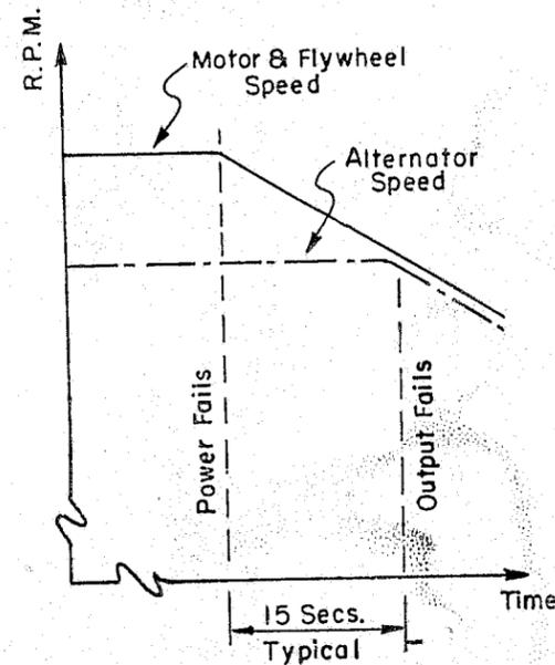
FIGURE 6. Typical motor-alternator set with flywheel energy storage.
