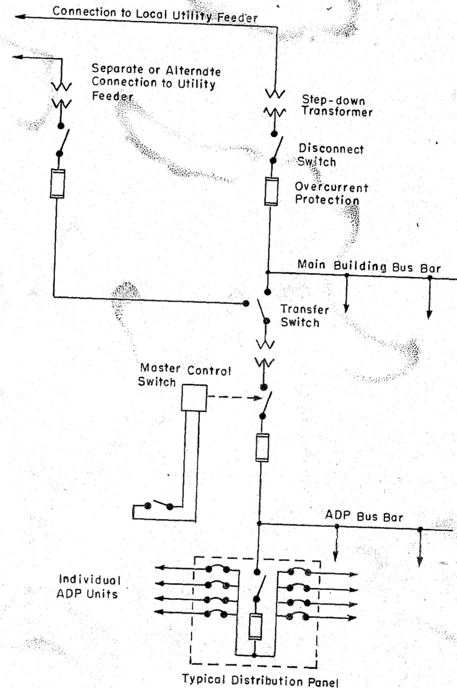
FIGURE 12. Simplified one-line diagram of power distribution.
