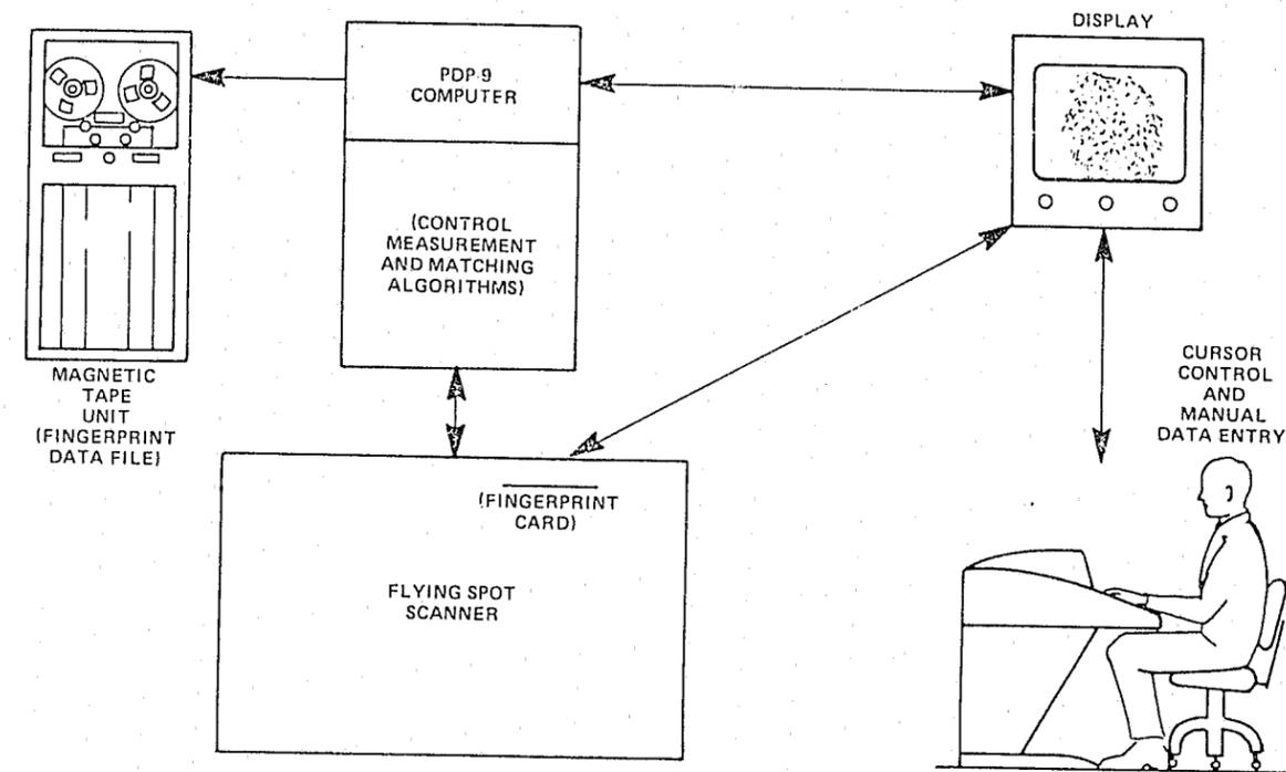
Figure 2 HARDWARE CONFIGURATION OF CALSPAN'S IMAGE PROCESSING LABORATORY FACILITY FOR THE FEASIBILITY DEMONSTRATION OF THE SEMI-AUTOMATIC FINGERPRINT READER
