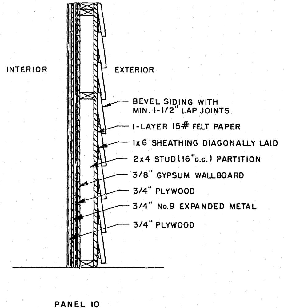
Figure 81. Construction of Panel 10
