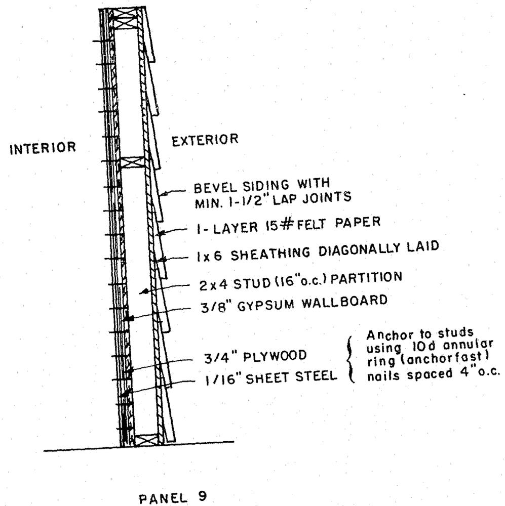
Figure 70. Construction of Panel 9
