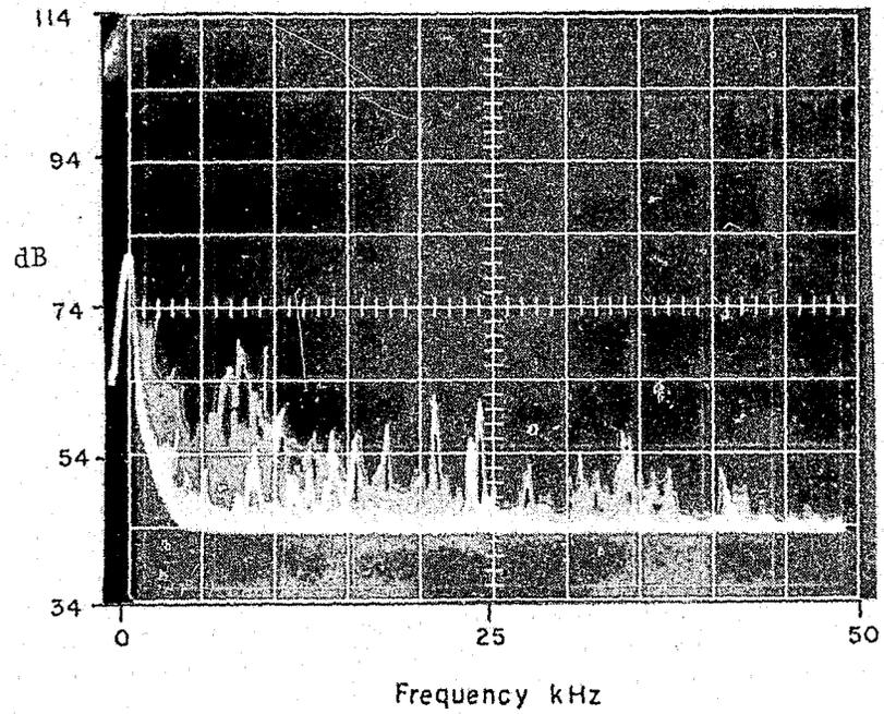
Figure 64. Acoustical Disturbances from Bolt Cutters; Test 8A
