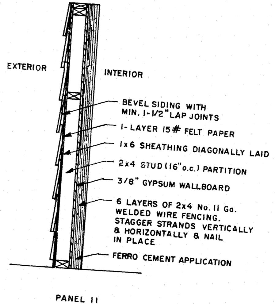
Figure 85. Construction of Panel 11
