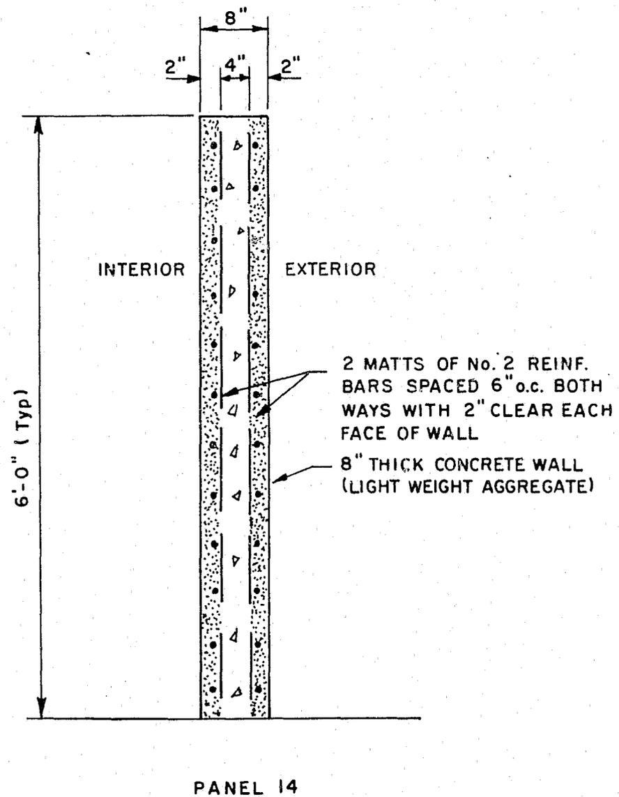
Figure 125. Construction of Panel 14
