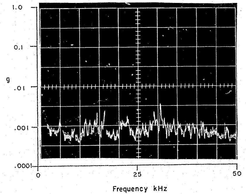
Figure 120. Test 13D. Vibrational Disturbances Produced by Burning Bar
