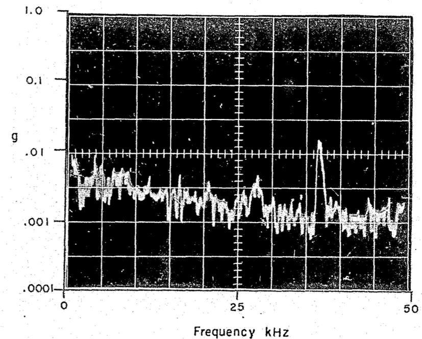
Figure 147. Test 16A. Vibrational Disturbances Produced by Torch
