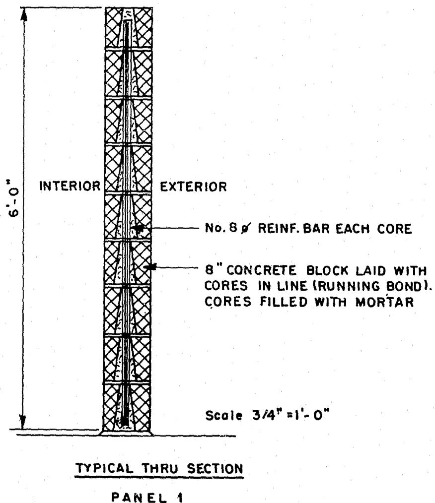
Figure 1. Construction of Panel 1
