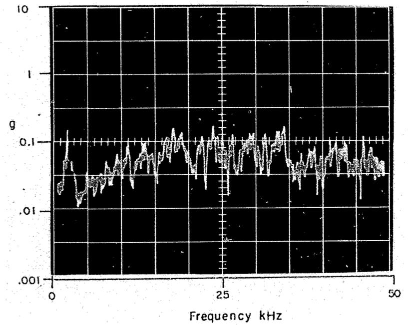
Figure 76. Vibrational Disturbances Produced by Abrasive Wheel Saw; Test 9M
