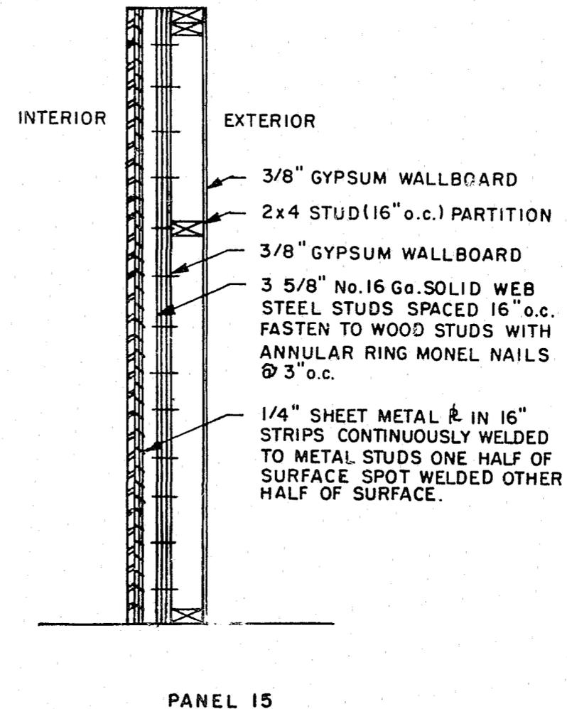
Figure 131. Construction of Panel 15
