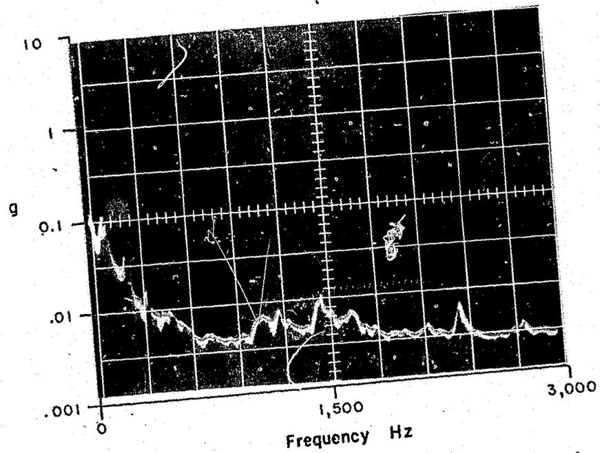
Figure 188. Vibrational Disturbances from 10' Fence Lifting and Man Crawling Under; Test F4
