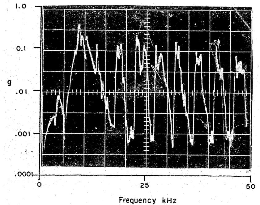
Figure 127. Vibrational Disturbances Produced by Rotohammer and Drill; Test 14B
