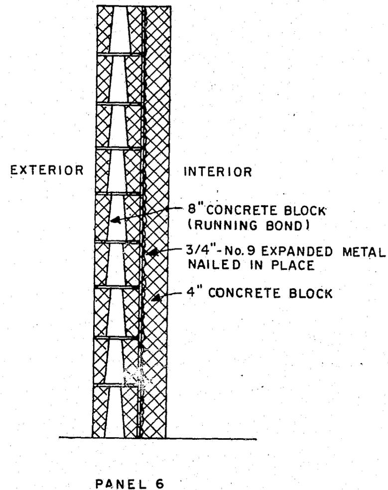
Figure 44. Construction of Panel 6
