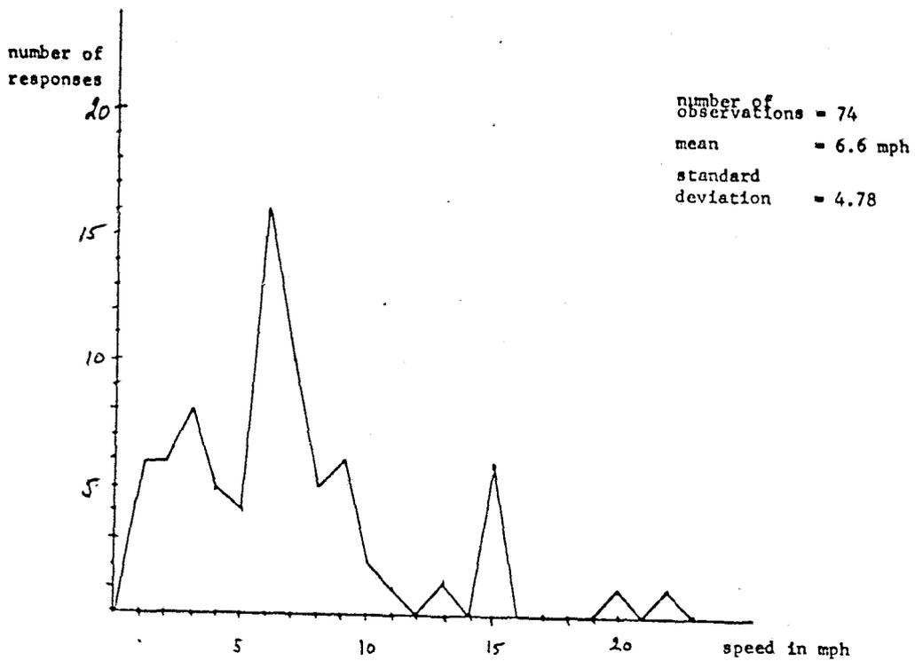
It is necessary to include this so that comparisons can be made with actual response times. The start-up time is set equal to 30 seconds. Fixing the return speed at 9.2 mph. and determining the response speed which yields the best response distribution fit to real data, yields 9.6 mph. and a start-up time of one minute (Chi-square is 6.00 for 15 degrees of freedom, which is significant at 2.5% level).
