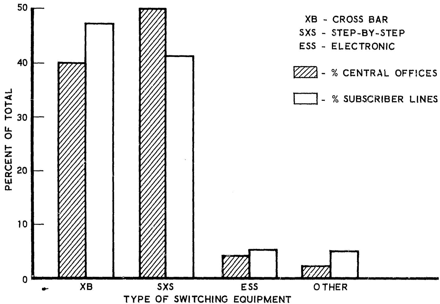
Figure 18. Distribution of Central Offices and Lines by Type of Switching Equipment - 1973
