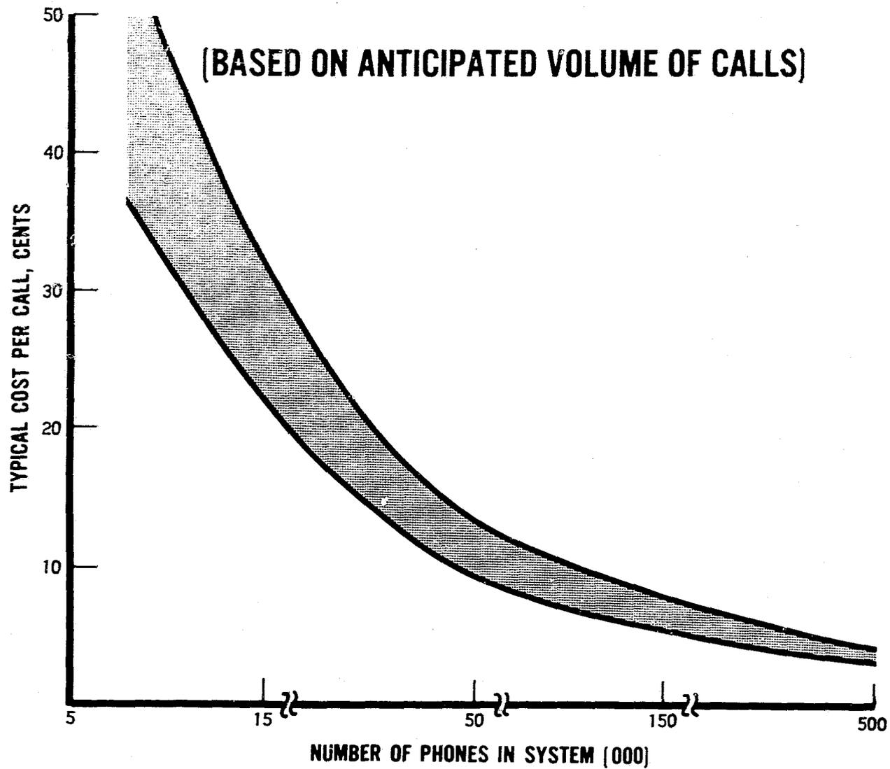
Figure 16. 911 ALI Hardware Cost Per Call as a Function of Size of Installation
