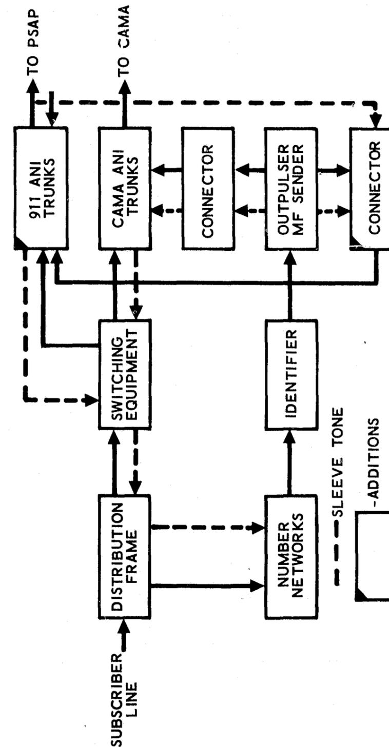
Figure 33. Modification to ANI-Equipped Offices
