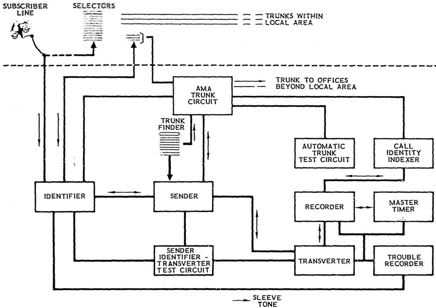
Figure 22. Automatic Message Accounting in Step-by-Step Offices
