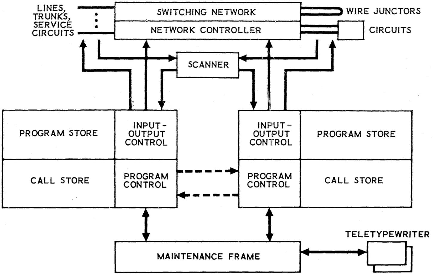
Figure 28. Electronic Switching System
