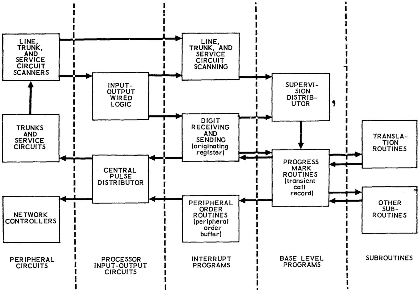
Figure 29. ESS Call Processing Information Flow
