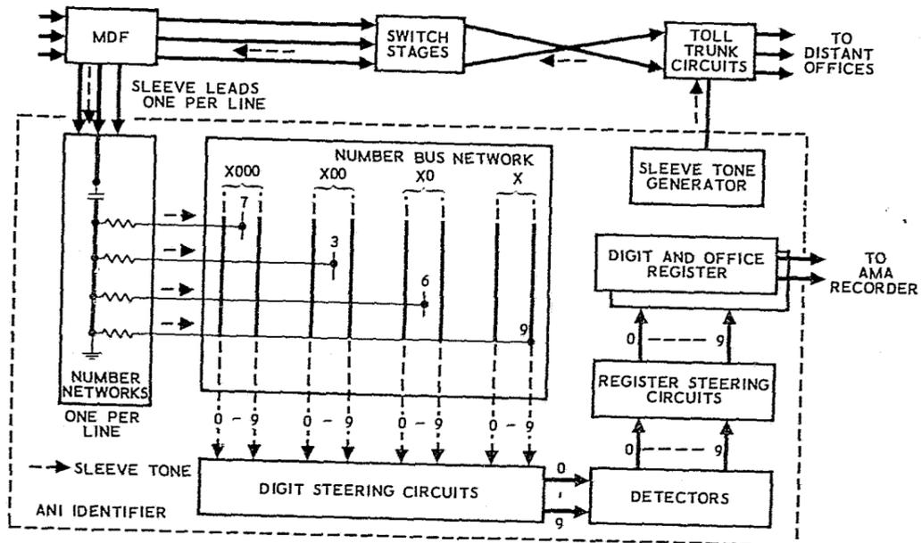
Figure 23. AMA Identifier. Typical Calling Number Identifier Circuit Used in Step-by-Step and No. 1 Crossbar Offices with AMA
