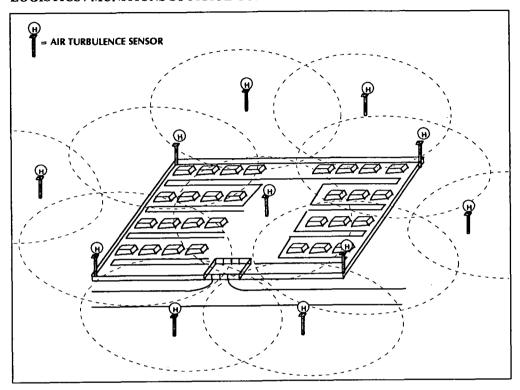
NOTE: The Acoustic Screen can be extended and configured to conform to the surrounding topography and potential approaching corridors, thereby increasing the "early warning" and positional location/axis of the intruding aircraft.
