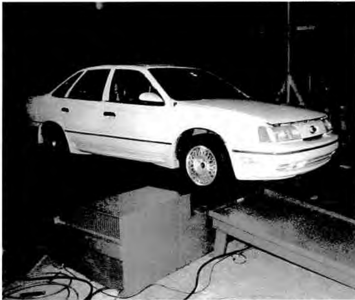
Photo 4. Vehicle mounted on dynamometer
