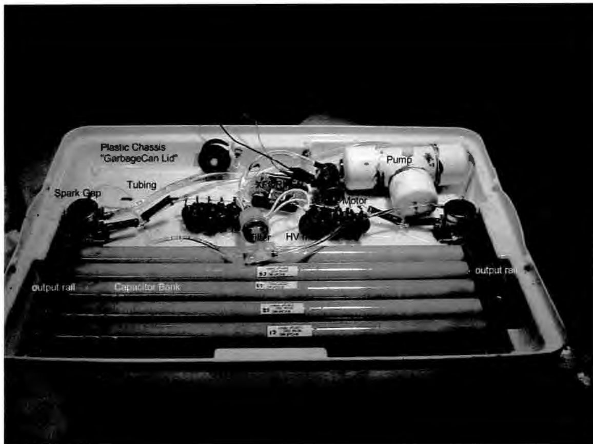
FIG 1 Road Sentry Prototype Chassis Assembly Showing Major Components:
