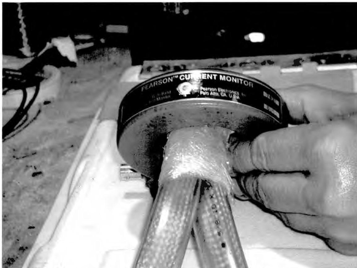
FIG 8 Showing Pearson Probe with HV Insulated Current Shunt
