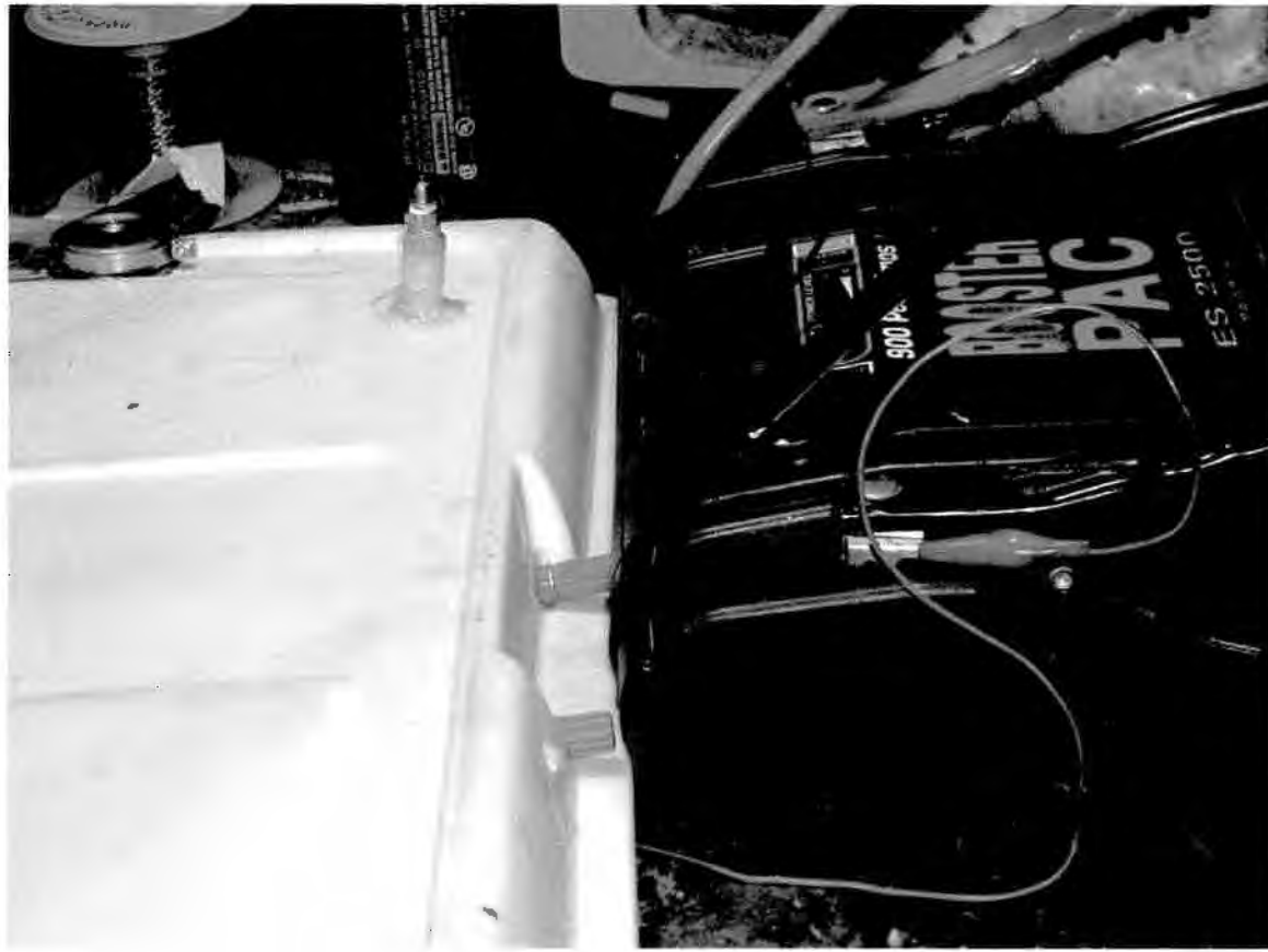
FIG 5 Showing 12VDC Connection for Internal Dielectric Pump Drive
