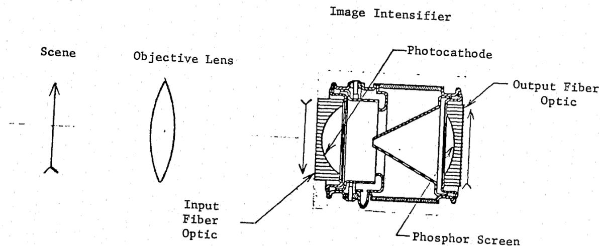
Fig. 2-1- Image Intensifier System Schematic
