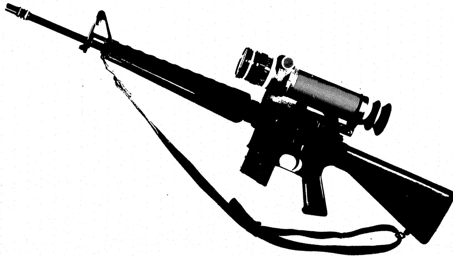
Fig. 3.2-2 GOEC MK 202 Mounted on M-16 Rifle
