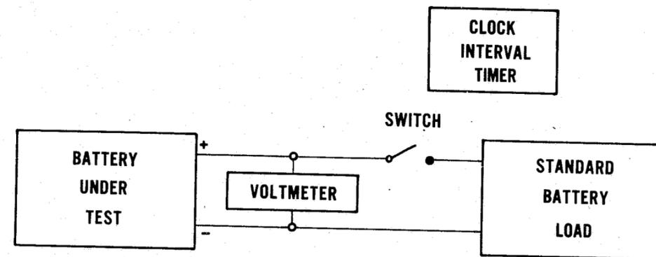
FIGURE 1. Block diagram for closed-circuit voltage test.
