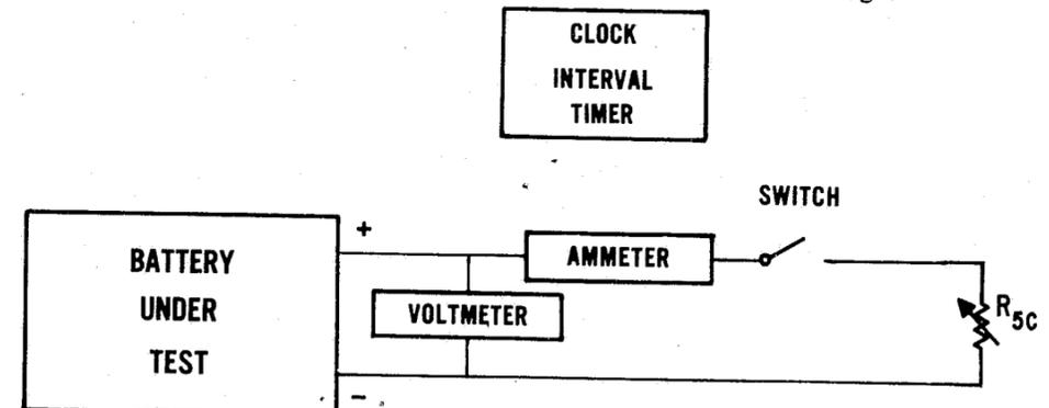
FIGURE 4. Block diagram for internal connection test.
