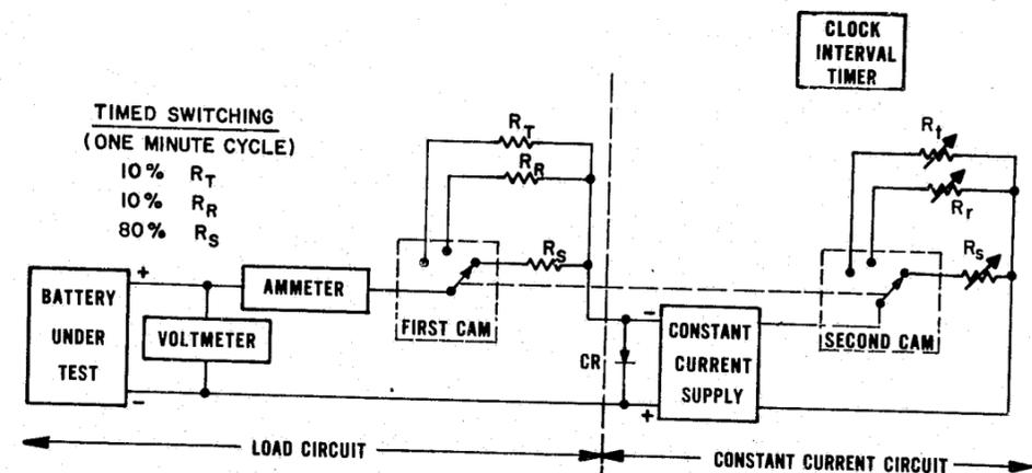
FIGURE 2. Block diagram for service life test.
