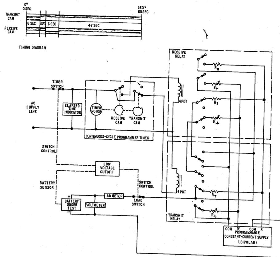
FIGURE 3. Wiring diagram for automatic service life measurements.
