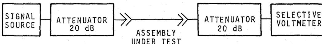
FIGURE 3. Block diagram for insertion loss measurement.
