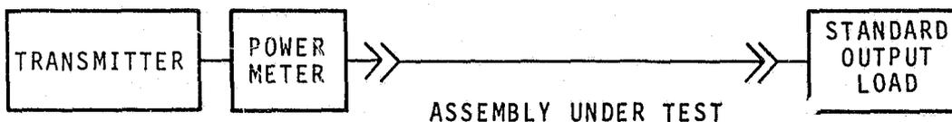
FIGURE 2. Block diagram for SWR measurement.
