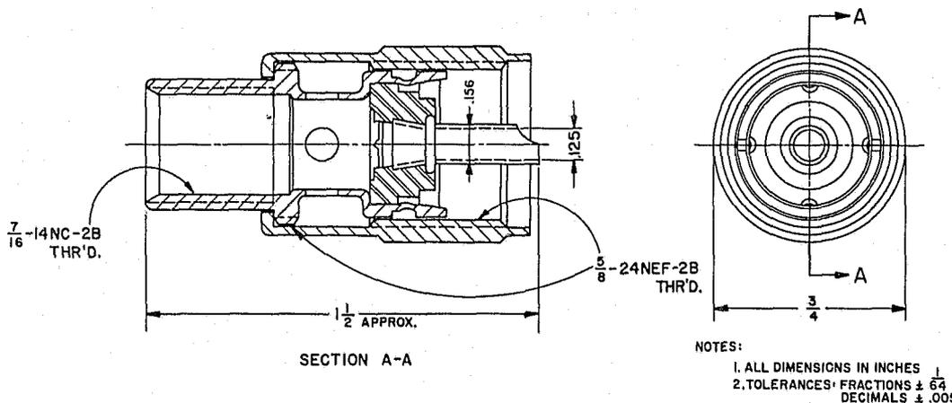
FIGURE 1. Connector plug.
