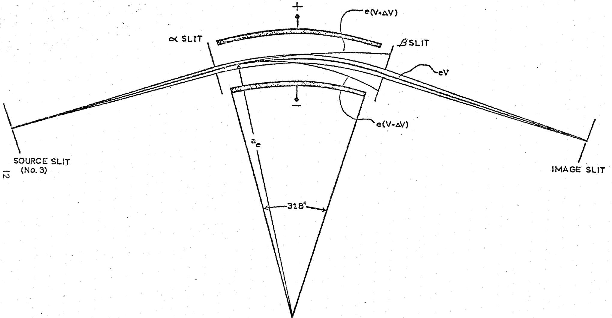
Figure 2. Electrostatic analyzer
