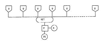
This is perhaps the simplest of CLIS configurations. All users would interface their terminals directly with a single-processor complex. This configuration also provides the greatest degree of centralized control.
