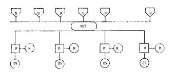
In this configuration all users have access to a common communications net and selective access to a processor complex depending upon the application area they are currently using.
