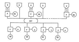
In this configuration certain high volume or specialized users will have dedicated local processor and data storage capability (using minicomputers) with multiple terminals. Other users will still be able to access the CLIS files using normal terminal operations. The communications network would become the central control point of the system.
