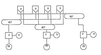
This system configuration provides for a communication network for each application area or groups of application areas. It also provides for distributed processing functions. Each user would have one or more terminals to connect to the selected application area.
