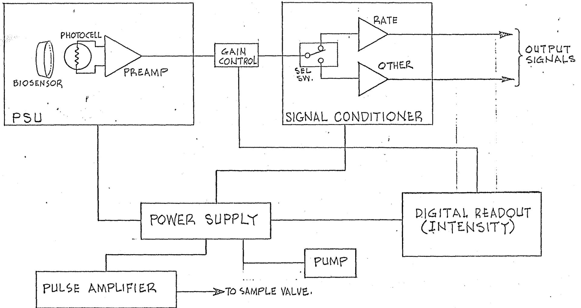
FIG. 4 ELECTRONIC SIGNAL PROCESSING
