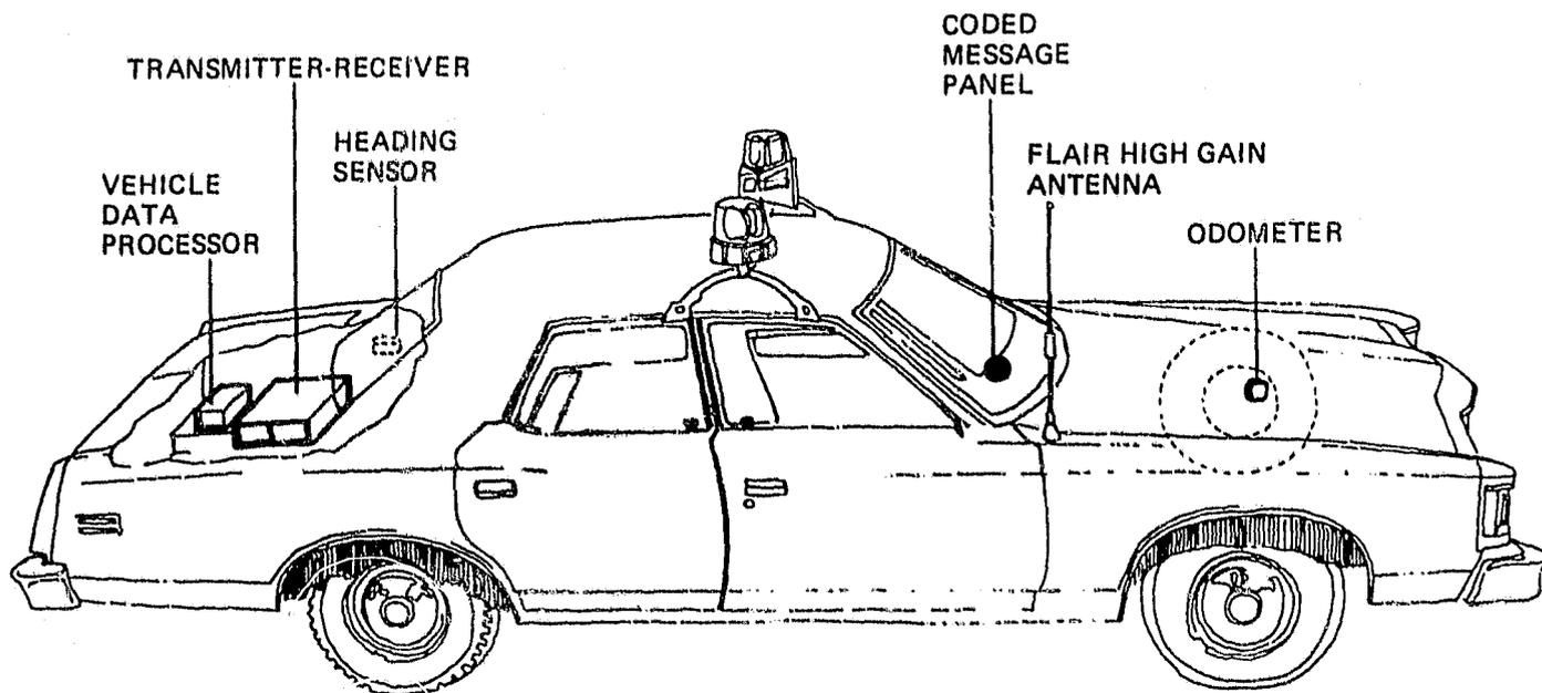
Fig. B-4. Typical mobile equipment installation
