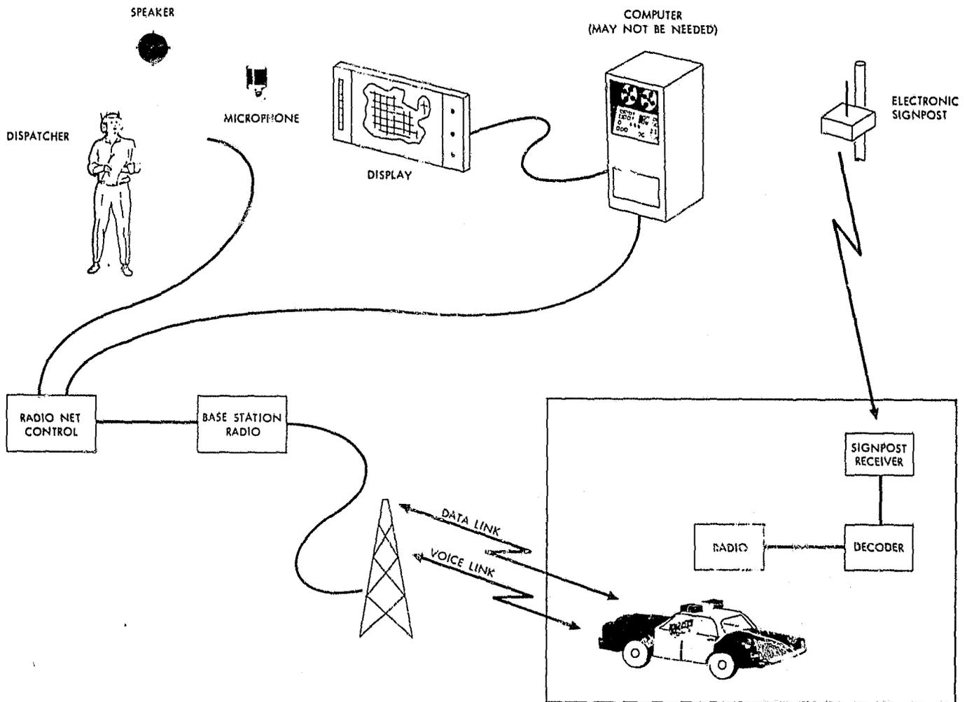
Fig. 4. Typical elements of a proximity AVL system
