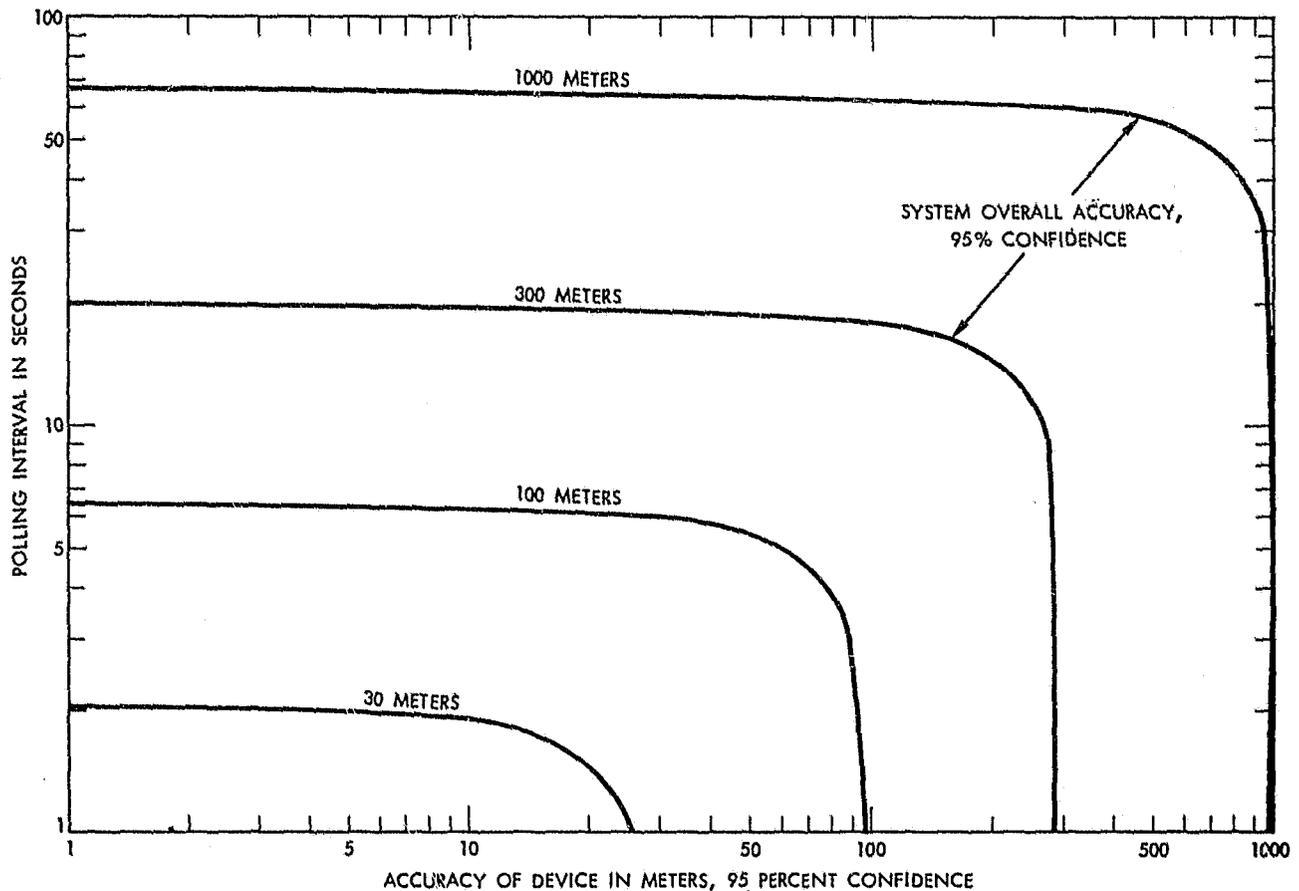
Fig. 10. AVL system accuracy
