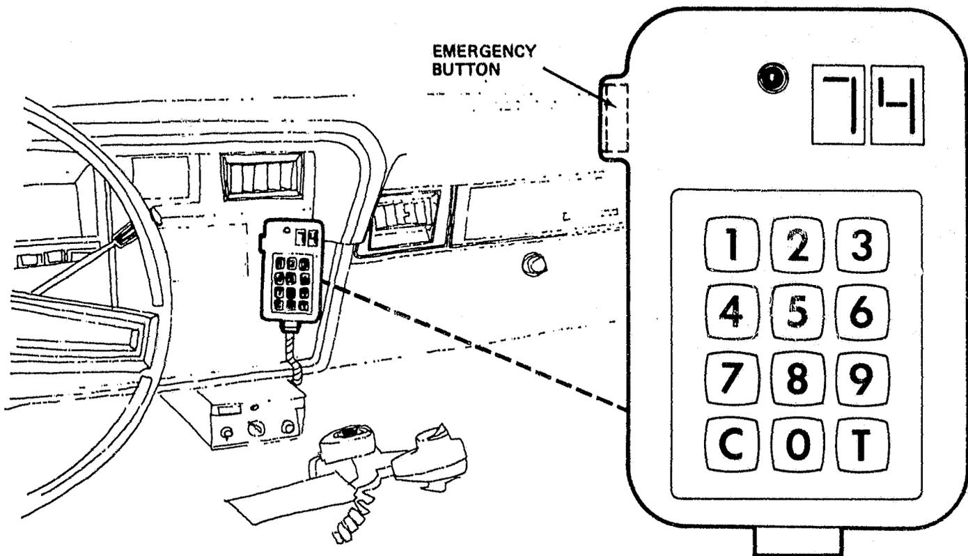
Fig. B-3. Typical coded message panel
