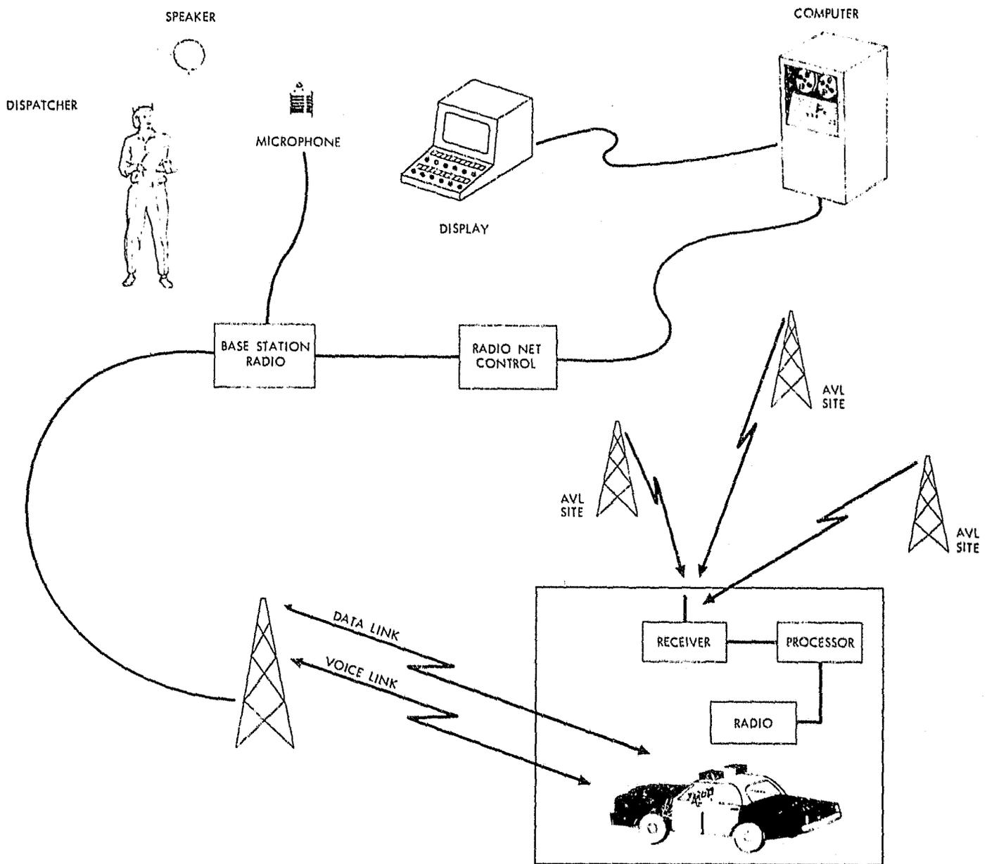
Fig. 7. Typical elements of a radiolocation AVL system
