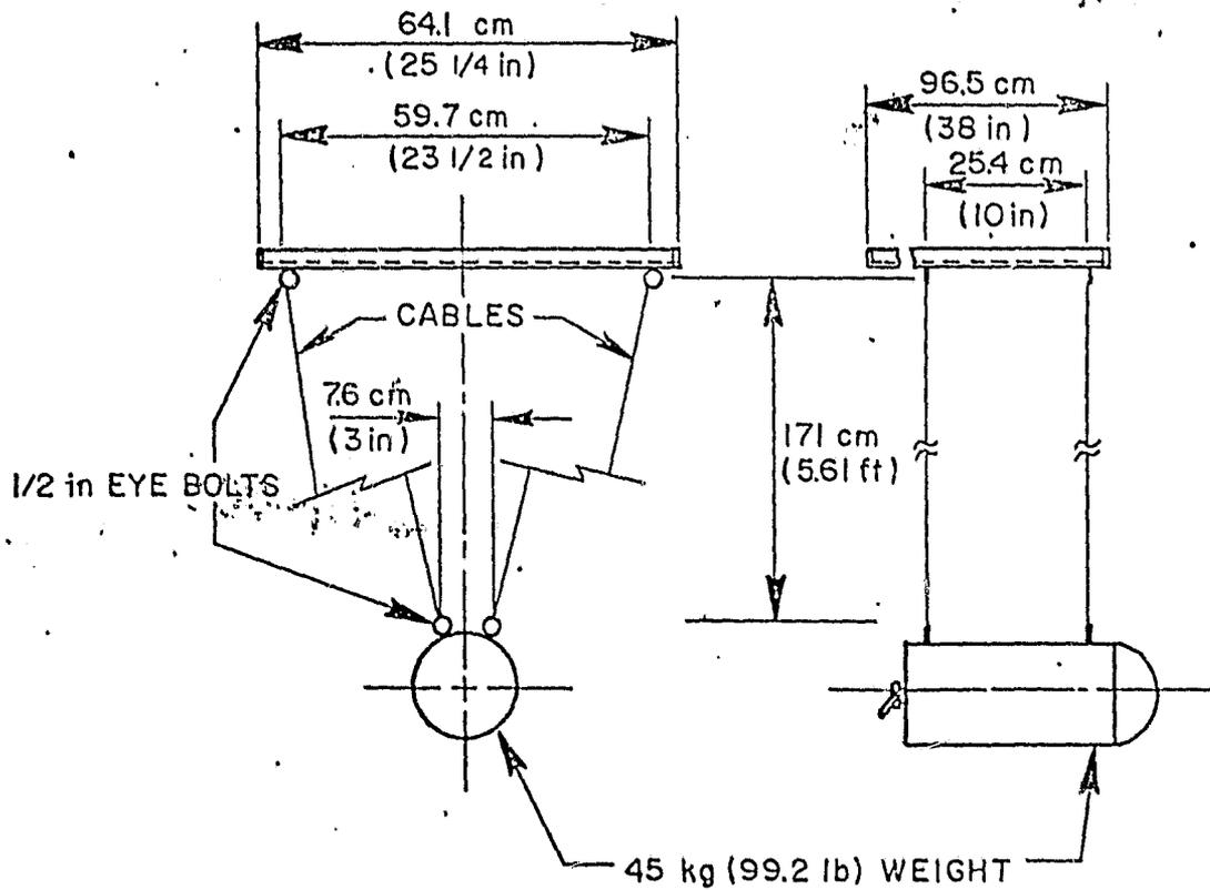
Figure B-3. Door Ram Suspension System
