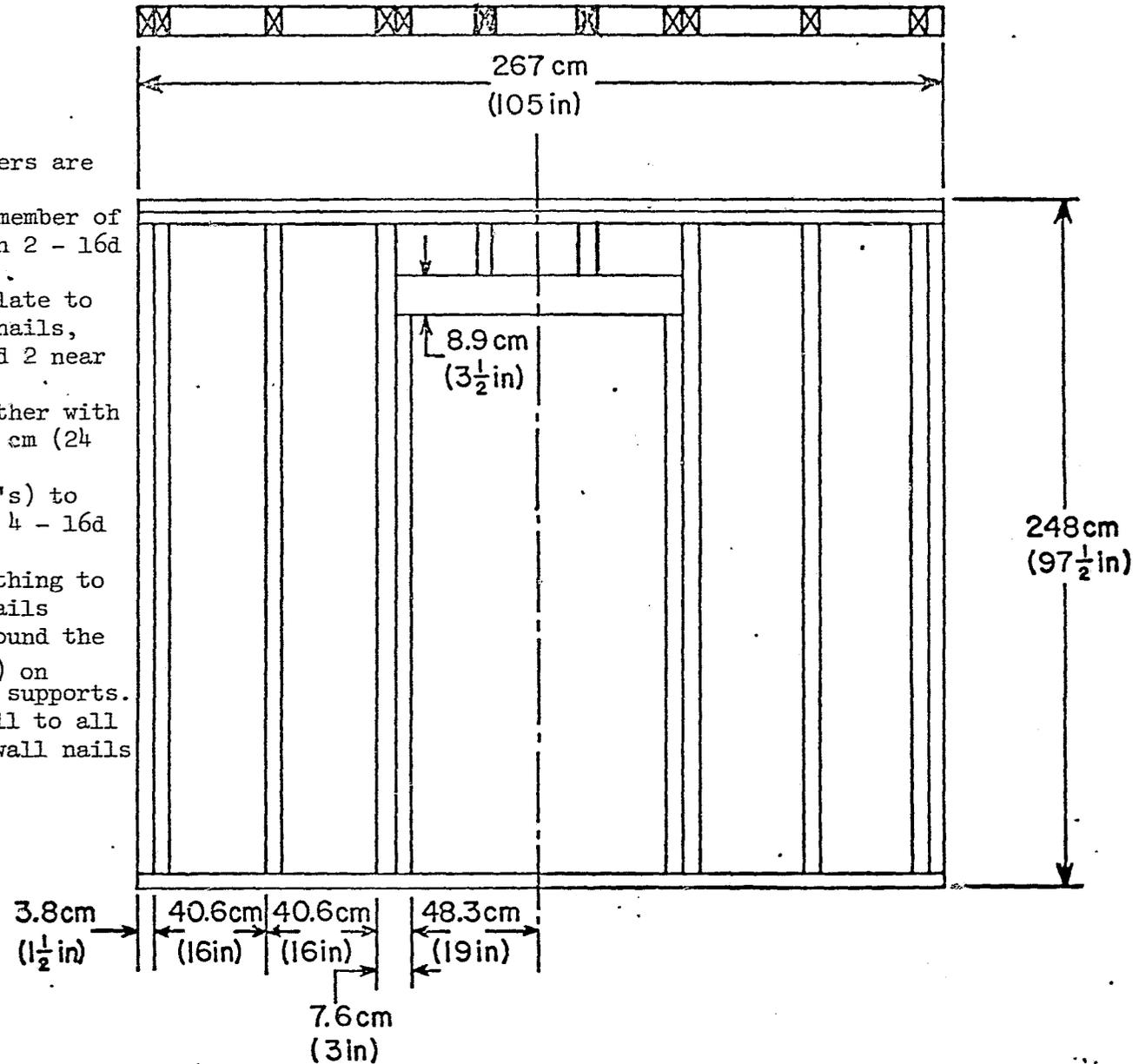
Figure 2. Door, Door Jamb, Hinge, and Lock Strike Component Fixture
