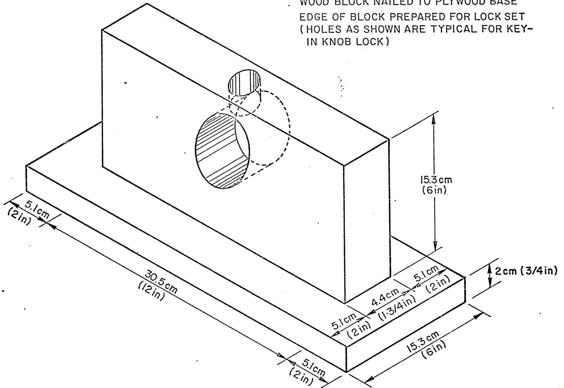
Figure 4: BOLT PRESSURE TEST FIXTURE
