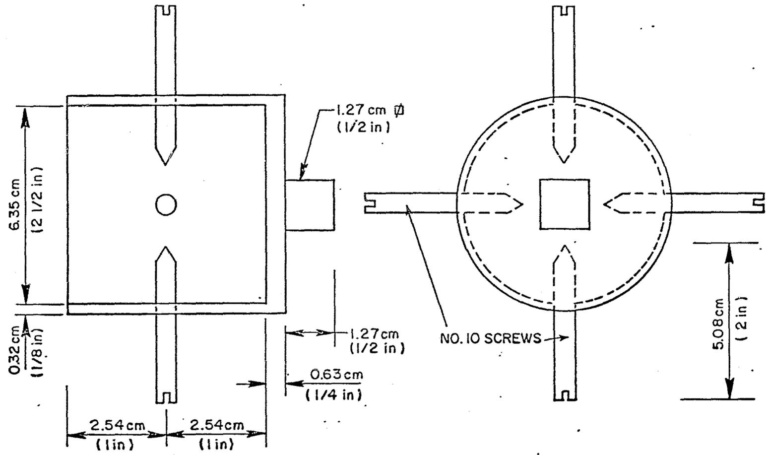
Figure B-9. Knob-Torque Adapter
