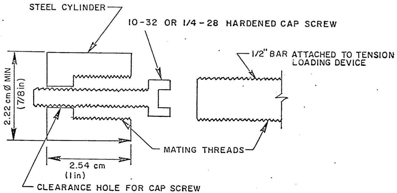
Figure B-12. Tension Loading Adapter
