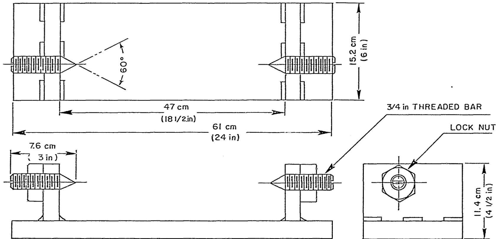
Figure B-7. Vertical Impactor Pivot Assembly
