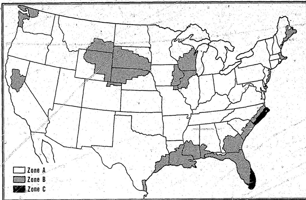
Figure 1. Location of wind loading zones based on 50 year mean recurrence interval.
