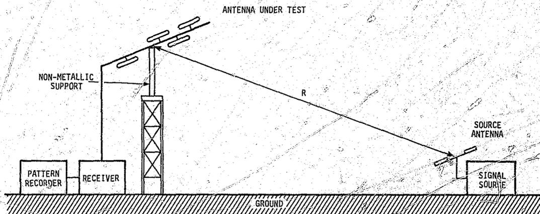
Figure 2. Test setup for measuring relative antenna gain and vertical radiation pattern.
