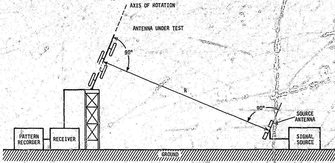
Figure 3. Test setup for measuring horizontal radiation pattern.
