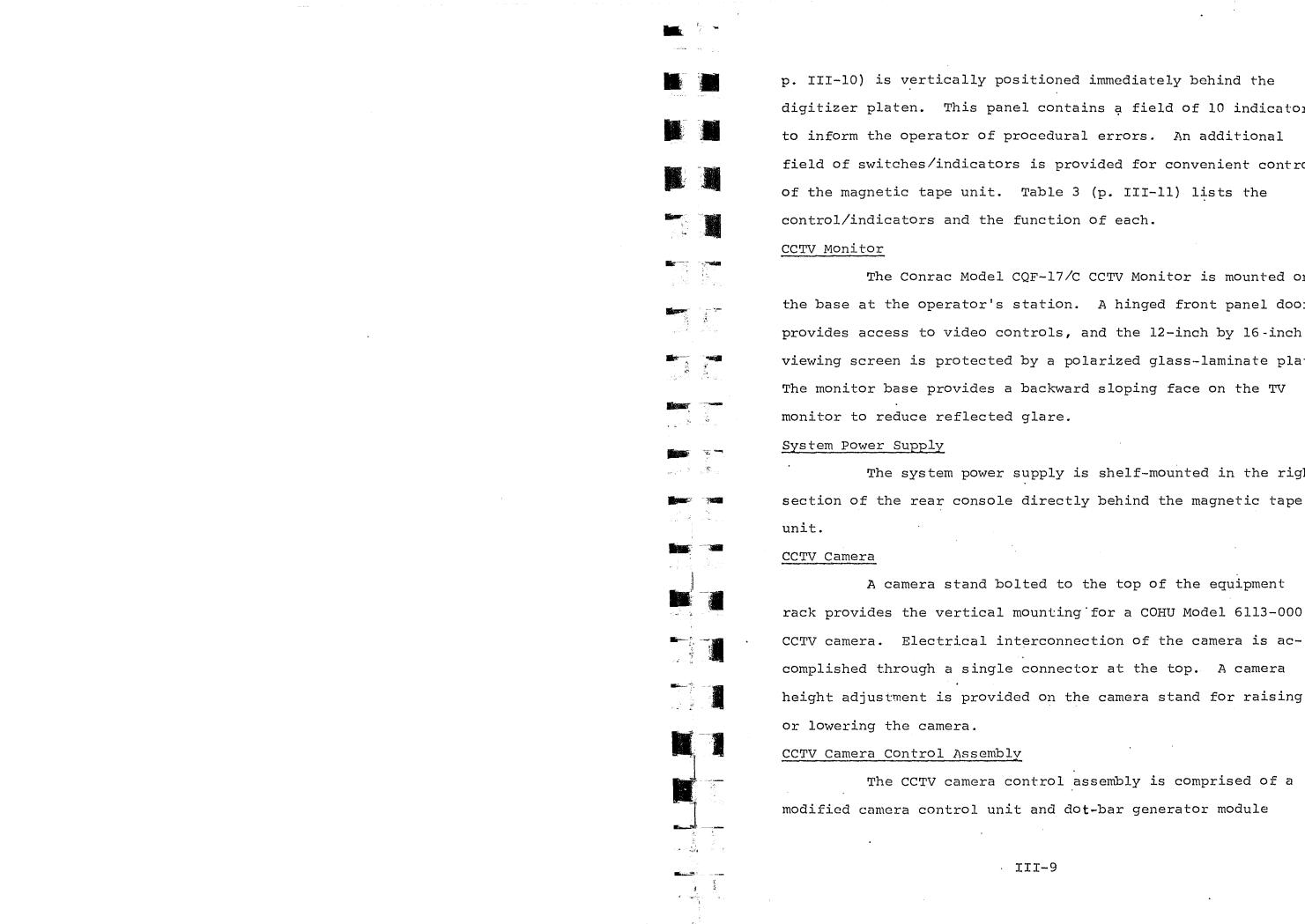
digitizer platen. This panel contains a field of 10 indicators to inform the operator of procedural errors. An additional field of switches/indicators is provided for convenient control
