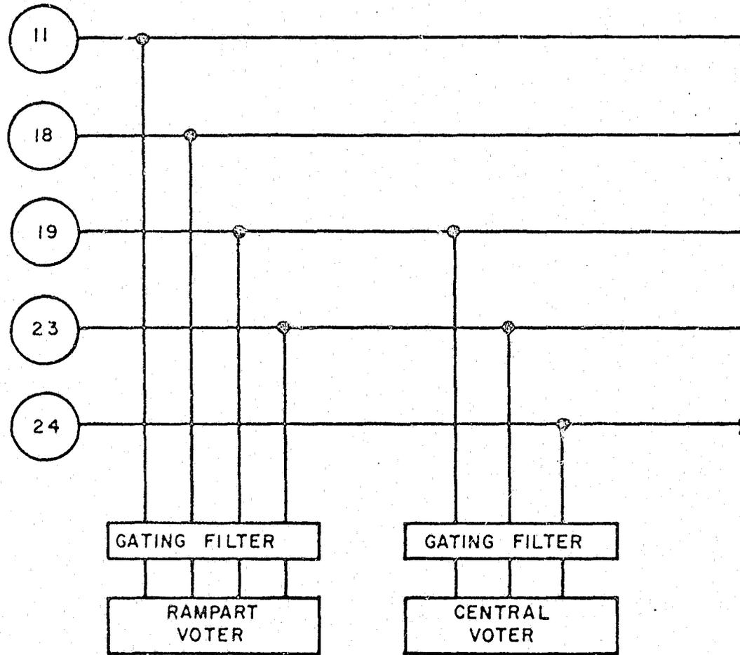
FIGURE 5-1 EXAMPLE OF MULTIPLE VOTING OF A SINGLE RF CHANNEL FOR RAMPART/CENTRAL AREAS
