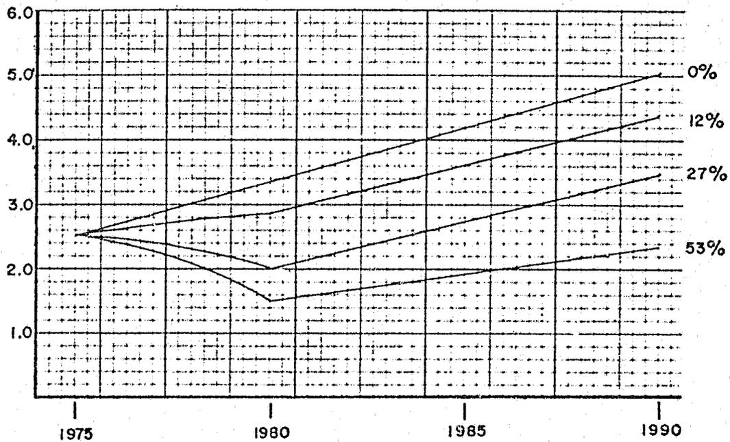
(a) DOWNLINK VOICE CHANNEL LOADING SENSITIVITY TO % OF DIGITAL TRANSMISSIONS
