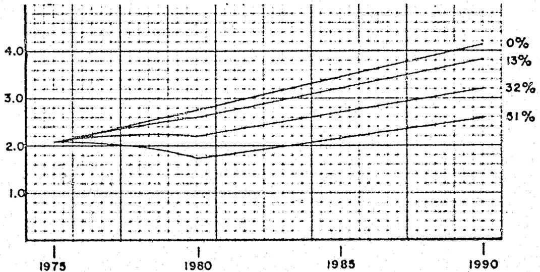
(b) UPLINK VOICE CHANNEL LOADING SENSITIVITY TO % OF DIGITAL TRANSMISSIONS
