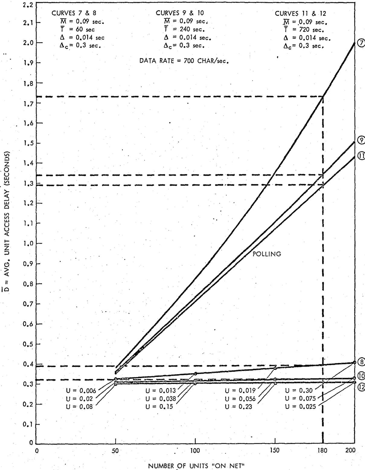
Fig. A-3. Relative Delays to be Expected in Either a Contention or a Polling System, Showing Curves 7, 8, 9, 10, 11, and 12
