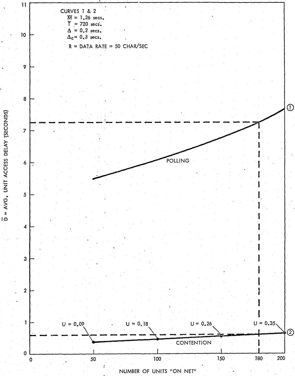
Fig. A-1. Relative Delays to be Expected in Either a Contention or a Polling System, Showing Curves 1 and 2
