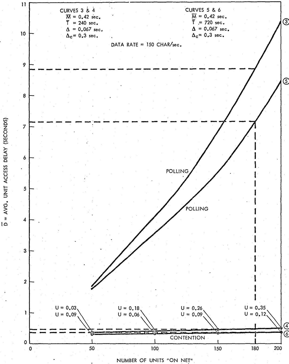
Fig. A-2. Relative Delays to be Expected in Either a Contention or a Polling System, Showing Curves 3, 4, 5, and 6
