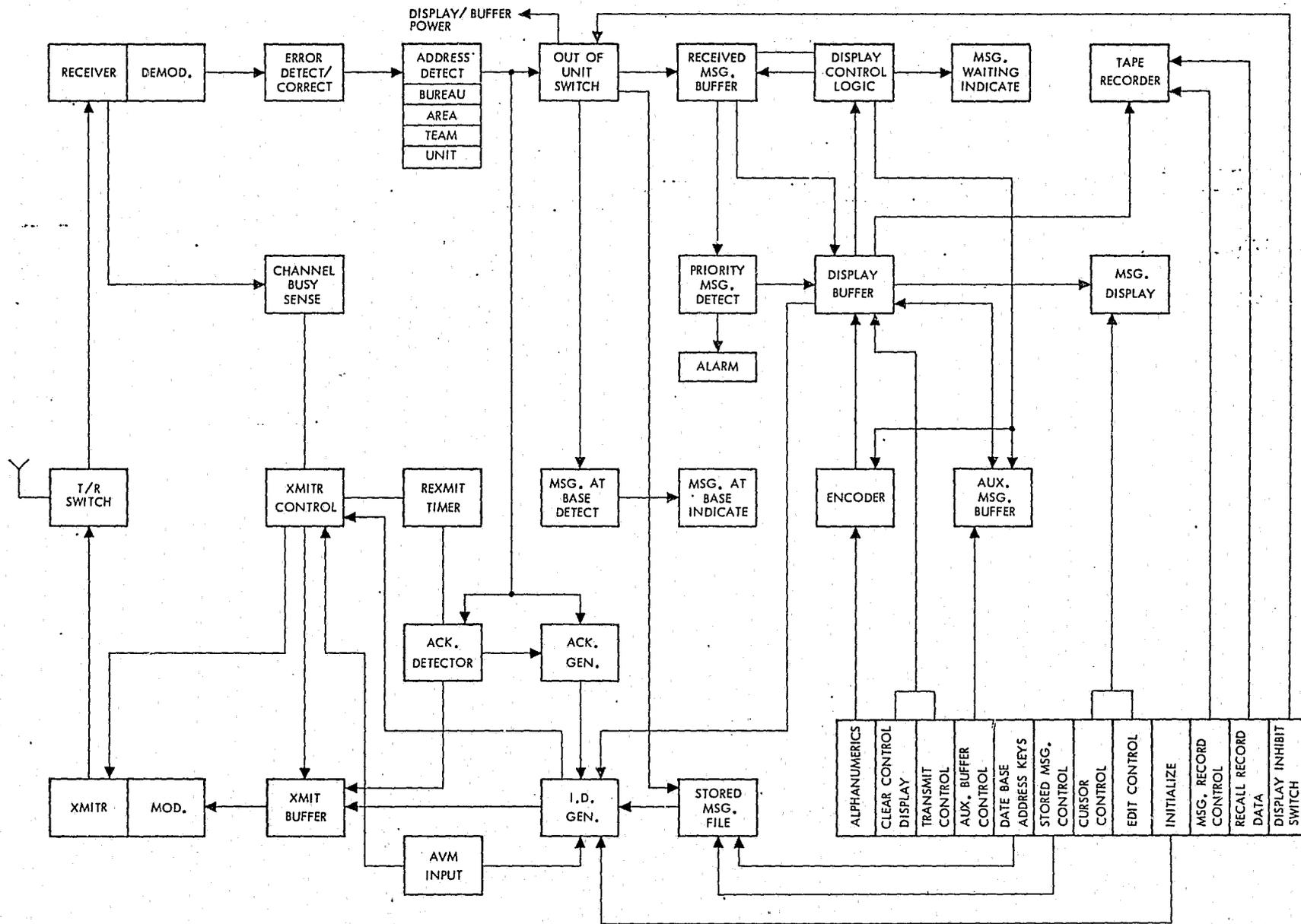
Fig. 3. ECCCS Phase I MDT Functional Block Diagram
