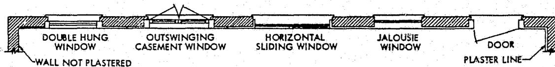
PLAN VIEW OF OPENINGS IN 8" BRICK WALL
