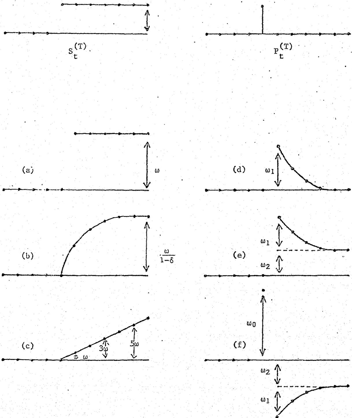
Figure 1. Six Basic Transfer Function Models
