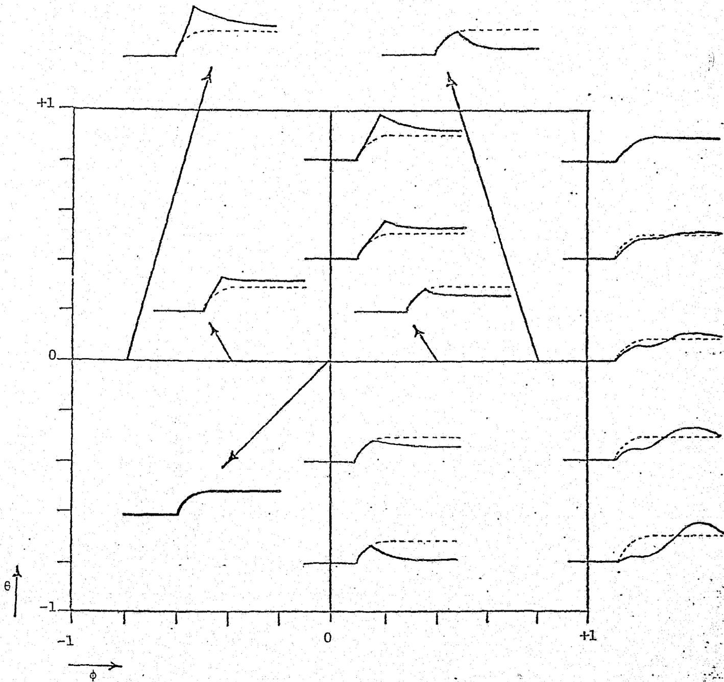
Figure 5. Effect of Variables  $M$  and  $\Lambda$  ( $\phi$  and  $\theta$ ) on the First-Order Step Response Model
