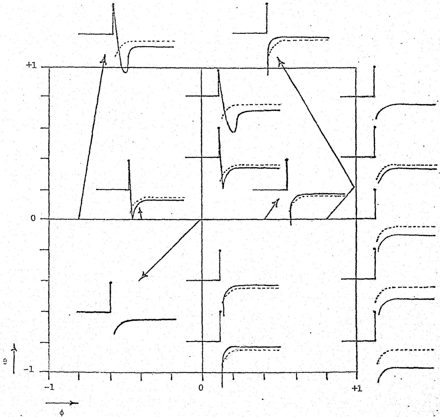
Figure 9. Effect of Variables  $M$  and  $A$  ( $\phi$  and  $\theta$ ) on the Inverse Decaying Pulse Response Model
