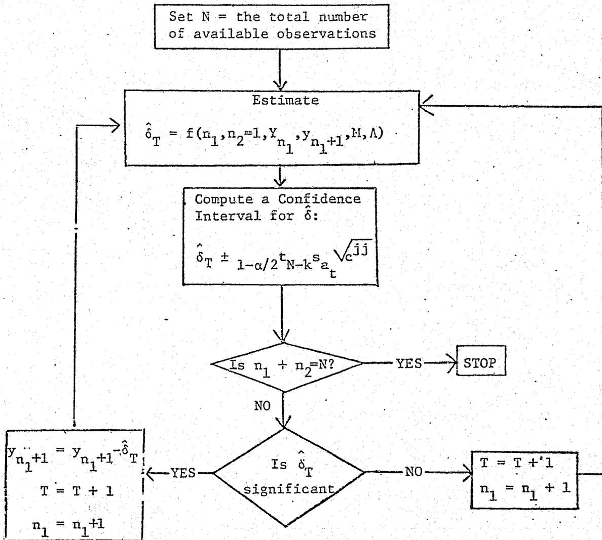
Figure 3. Flowchart for Identification Algorithm
