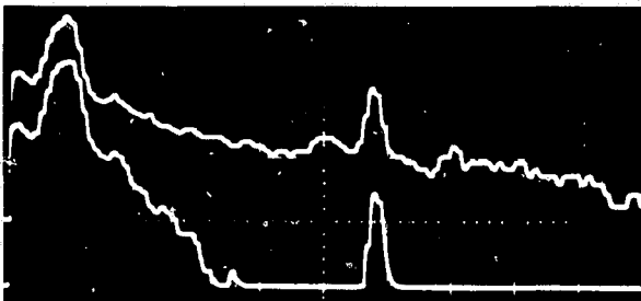
FIGURE 2. Left) Spectral plots with Right) 60 Hz filter out.
