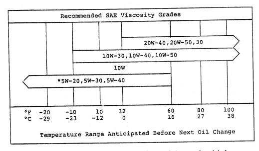
\*SAE 5W-20 NOT recommended for sustained high speed vehicle operation.
