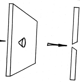
B. By an examination of stress lines on radial cracks near the point of impact, the direction of the force used to break the glass can be determined.
