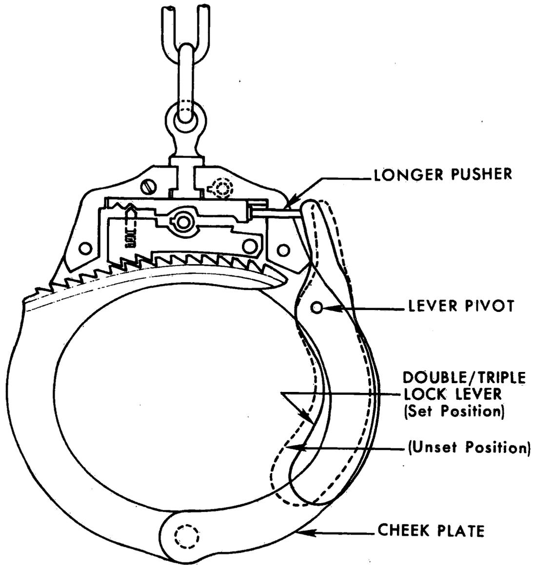
Figure 6. Partial cross section of improved handcuff with the double lock bolt inactive.
