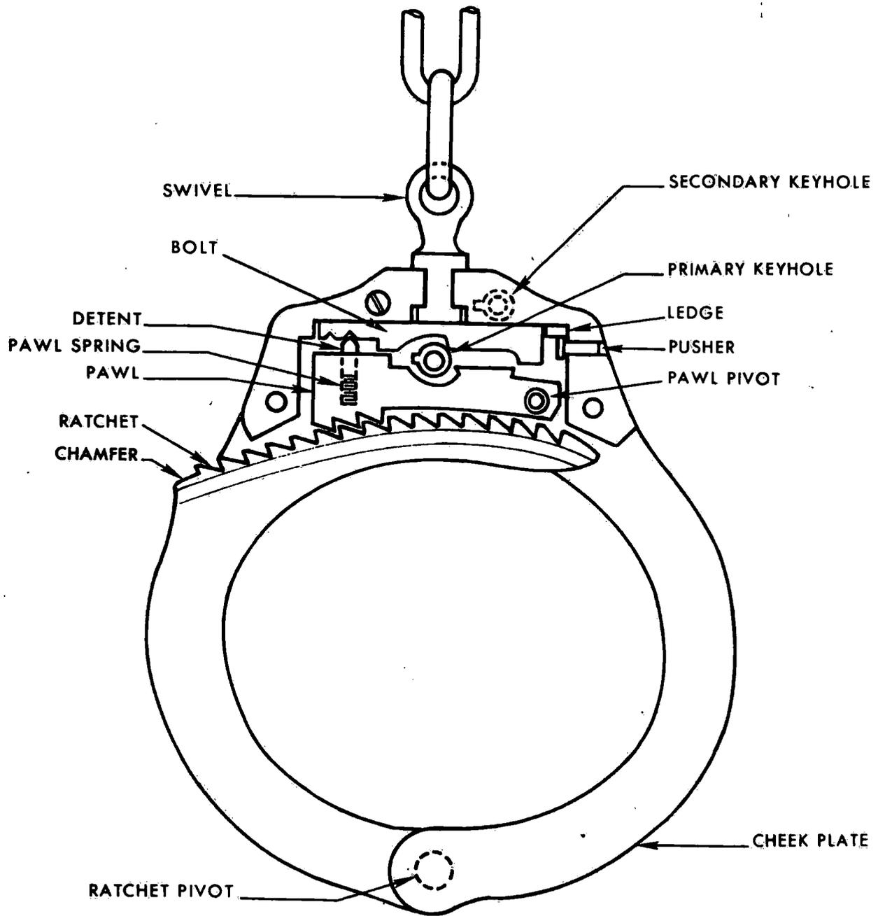
Figure 4. Partial cross section of a modified handcuff showing the secondary keyhole for unseating the double lock bolt and the chamfer of the last tooth of ratchet.
