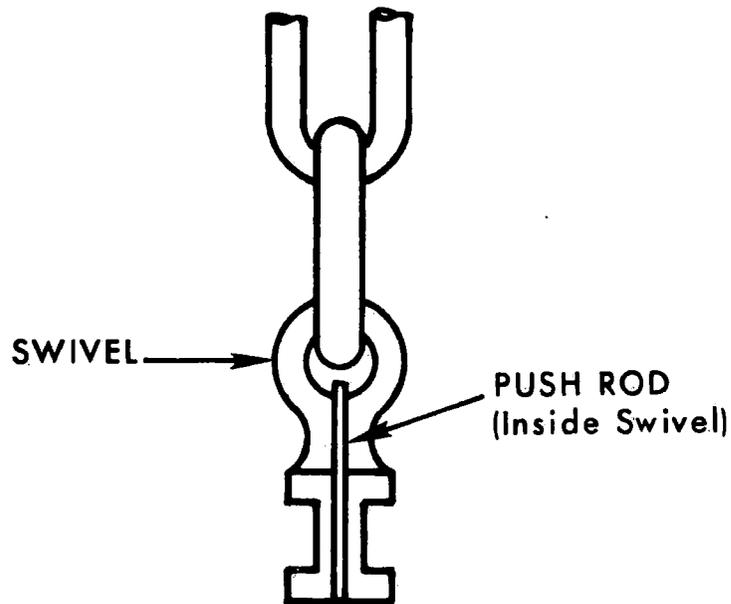
Figure 5. Alternate method of unseating an active double lock bolt.
