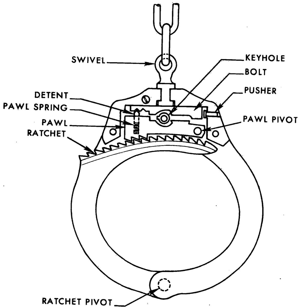
Figure 1. Partial cross section of a typical handcuff with the double lock bolt in the inactive position.
