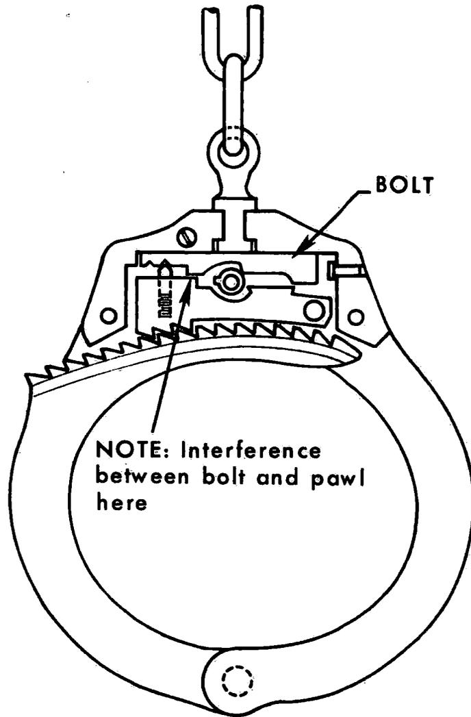
Figure 2. Partial cross section of a typical handcuff with the double lock bolt in the active position.
