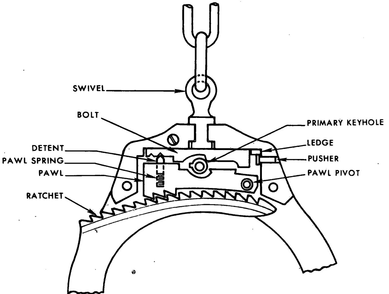
Figure 3. Cross section of a modified handcuff with the double lock bolt active and held in place by a locking ledge.
