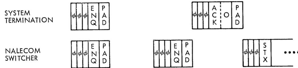
Fig. A-1. Transmission control sequences
