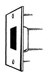
Replace weak strike plate with High Security Strike Plate. Fasten with long screws. This will also strengthen the frame system.
