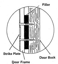
Replace screws with 21/2" screws. This will also strengthen the frame system.
