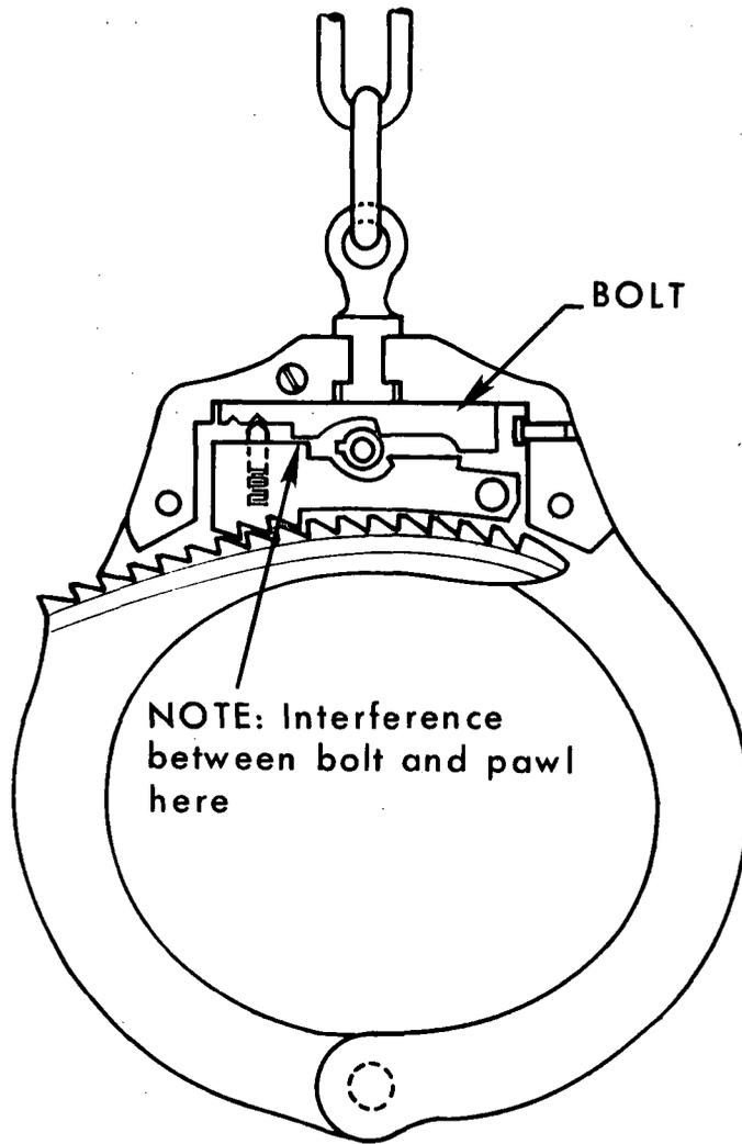
Figure 2. Partial cross section of a typical handcuff with the double lock bolt in the active position.
