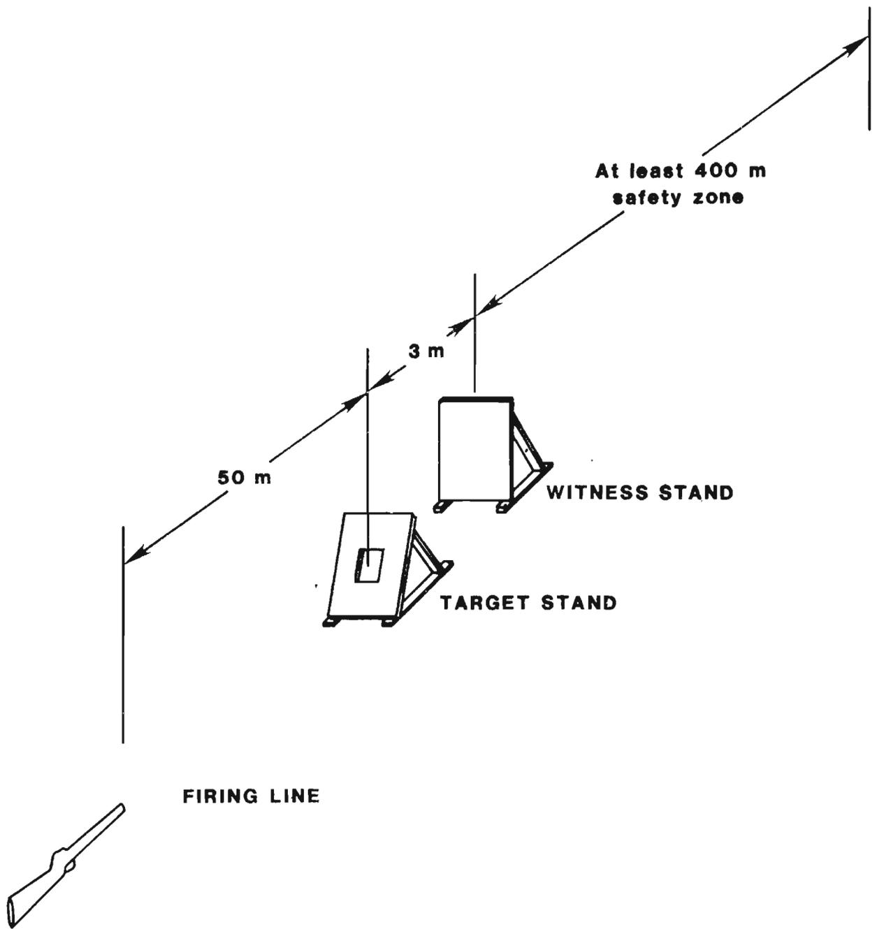
FIGURE 4. Penetration test setup.
