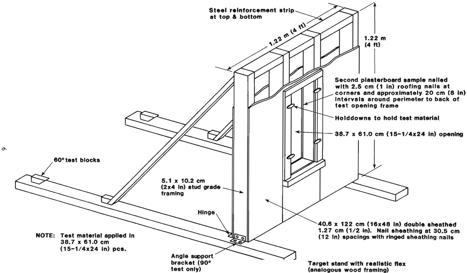
FIGURE 1. Penetration test target support.
