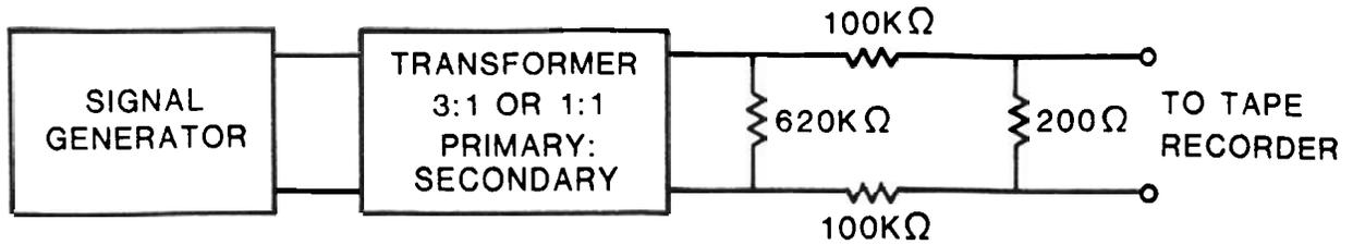
FIGURE 4. Block diagram for transformer circuit used in the microphone input, record-level indicator, overall frequency response, signal-to-noise ratio, interchannel crosstalk ratio, and recorded tape protection measurements.
