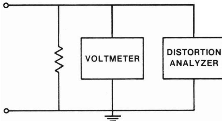
FIGURE 5. Block diagram for circuit used in the harmonic distortion measurements.
