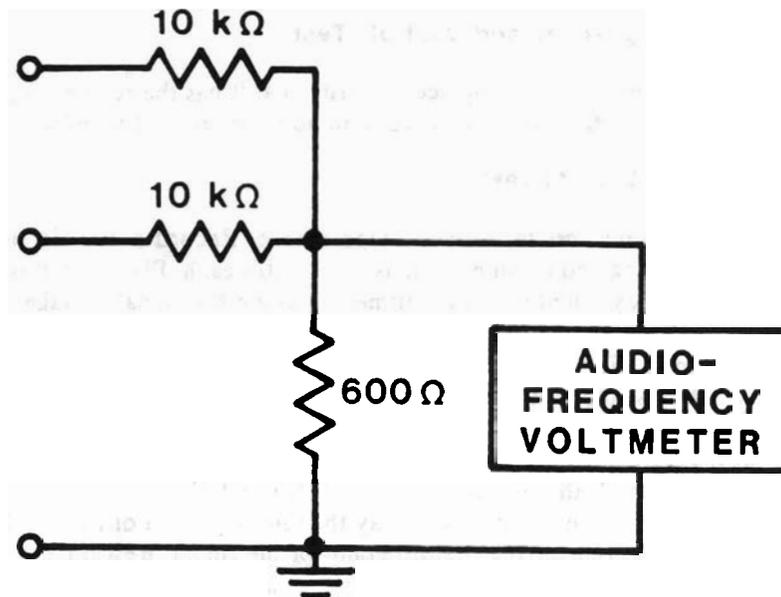
FIGURE 3. Block diagram for circuit used in the playback phase, record phase and track format measurements.
