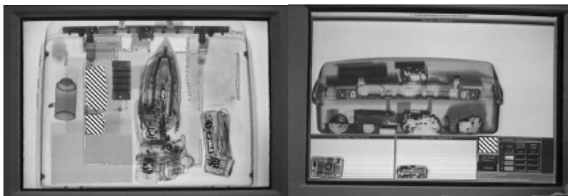
Figure 13. Dual energy system images rendered in black and white. The image on the left is from the vivid VDSI (stripes indicate the presence of contraband), and the image on the right is from the EG&G/Astrophysics Z-Scan (striped alarm square in the lower right hand corner indicates presence of contraband.)
