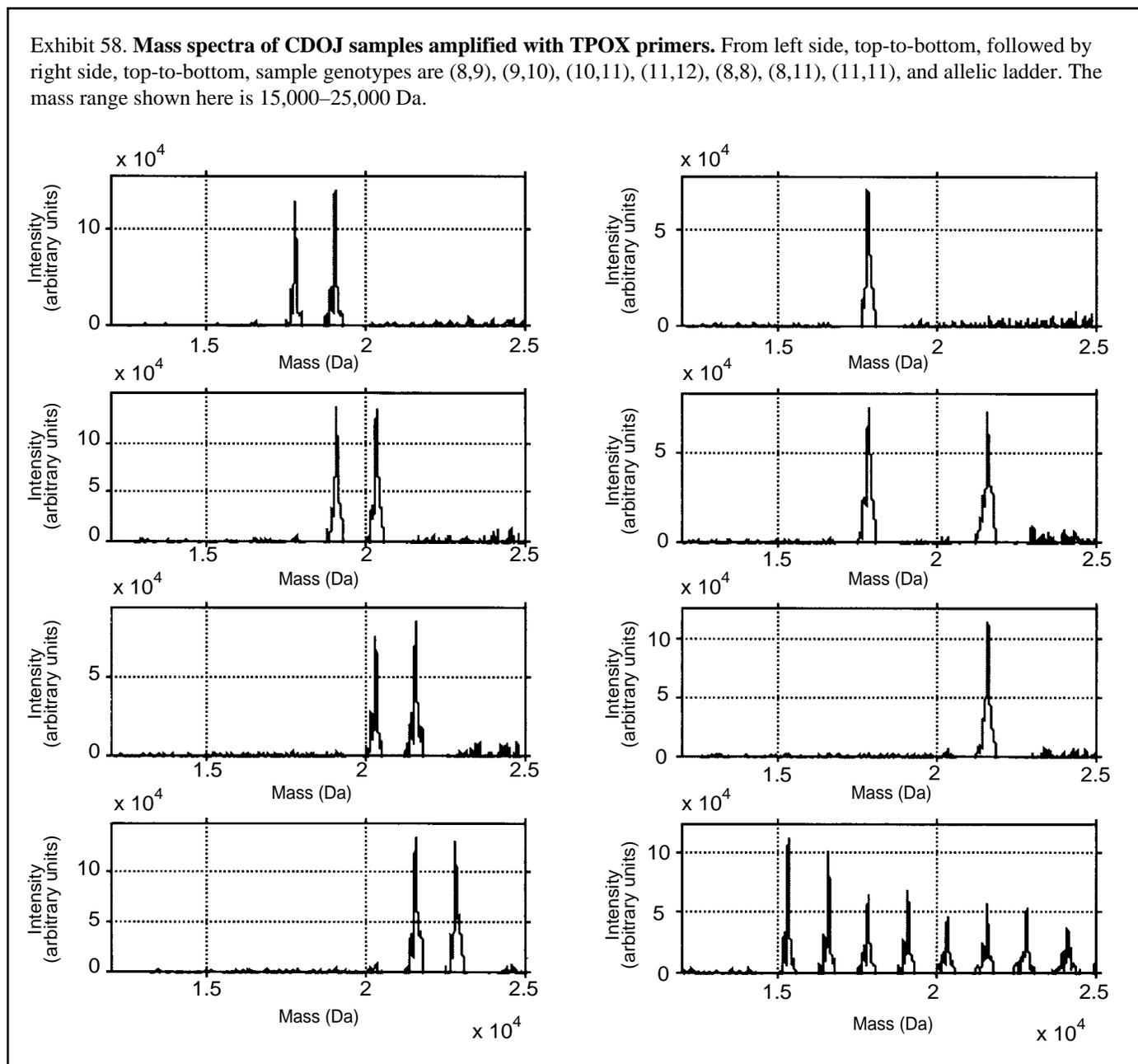
Precision is important for STR allele measurements in mass spectrometry because no internal standards are being run with each sample to make adjustments for slight variations in instrument conditions between runs. To demonstrate the excellent reproducibility of mass spectrometry, 15 mass spectra of a TPOX allelic ladder were collected. A table of the obtained
