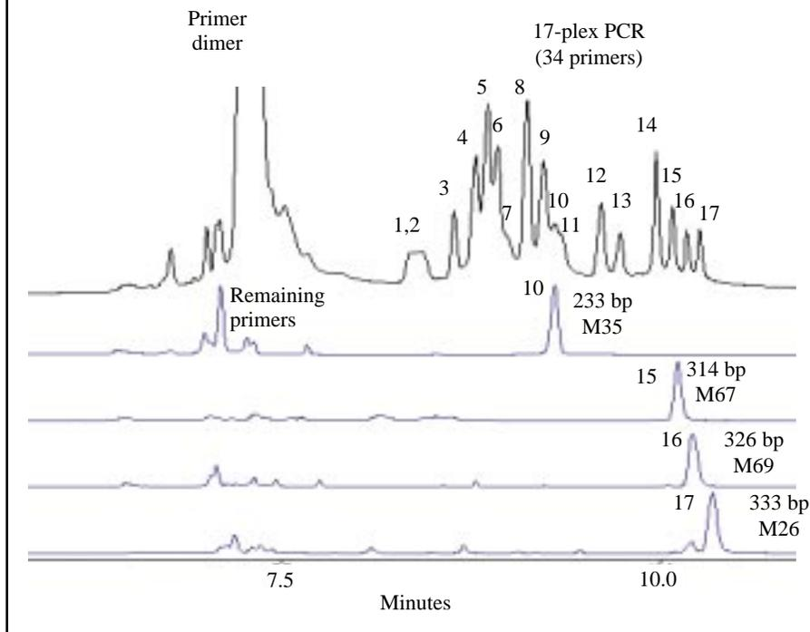
Exhibit 69. **Primers for testing Y-chromosome SNP markers in singleplexes.** Primers were designed automatically with UNIX SNP probe scripts written by Nathan Hunt but have not yet been tested.
