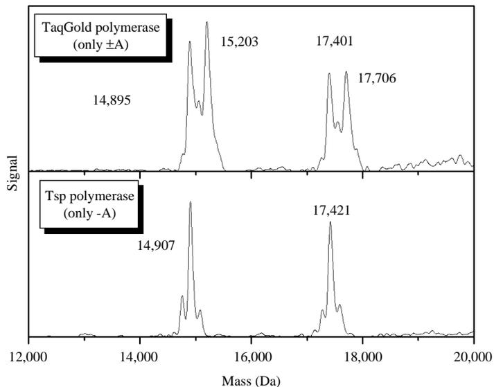
**Exhibit 49. Mass spectrum demonstrating detection of stutter products from a particularly stutter-prone dinucleotide repeat locus.** The mass differences between the stutter product peaks and the allele peaks can be used to determine the repeat sequence that is present on the measured DNA strand. Note: The amount of stutter is larger in the longer repeat allele than in the shorter allele.
