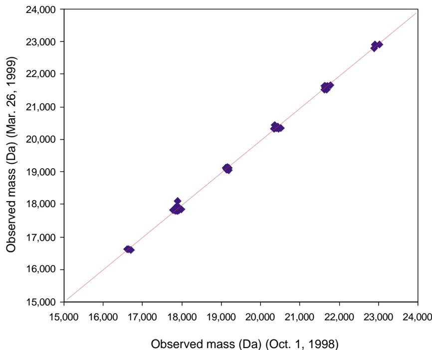
measurements from 6 different TPOX alleles collected 6 months apart. The first data set was collected on October 1, 1998, and the second data set on March 26, 1999. Amazingly enough, some of the alleles had identical measured masses, even though different mass calibration constants (and even different instruments) were used.
