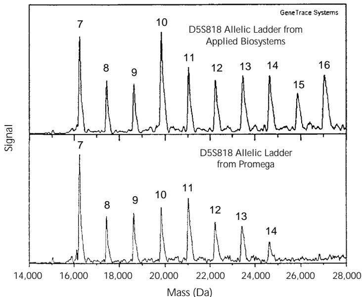
The analysis of STR allelic ladders demonstrates that all alleles can be resolved for an STR locus. Allelic ladders from commercial kits were typically diluted 1:1000 with deionized water and then reamplified with the
