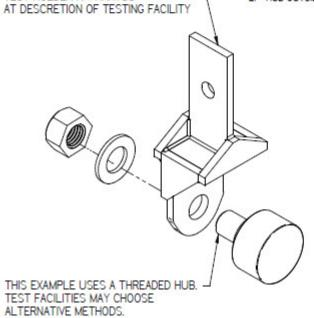
TEST HOLDER APPARATUS
