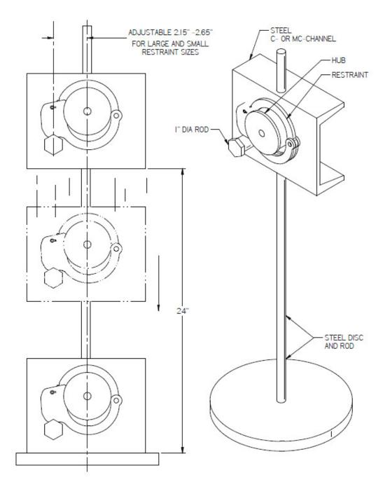
**Figure 17. Compression Test Setup**
