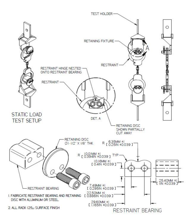
TEST HOLDER -RETAINING FIXTURE -RESTRAINT -RESTRAINT RESTRAINT BEARING SEE FIG. IT FOR DIMENSIONS RETAINING DISC Ø1-1/2" X 1/8" THK
