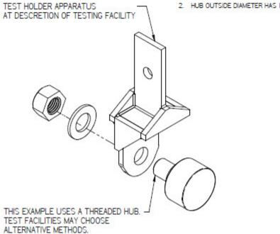
Figure 9. Double Loop Static Load Test Setup
