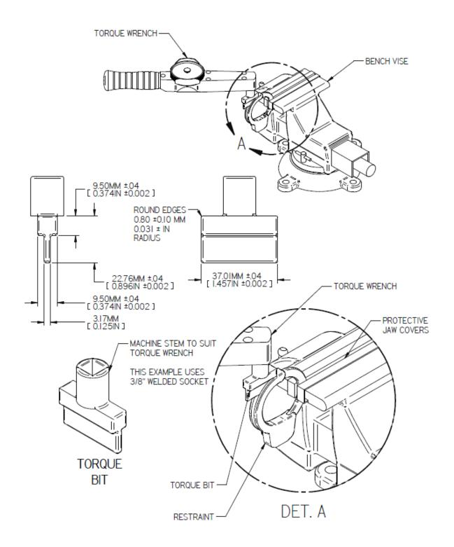
Figure 16. Double Lock Impact Test Setup
